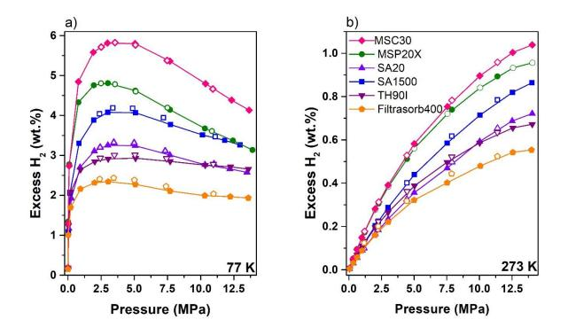
**Figure 2.** Excess hydrogen isotherms: (a) at 77 K; and (b) at 273 K, for the 6 CACs. Filled and empty symbols correspond to adsorption and desorption data, respectively, and the legend in (b) also applies to (a).
