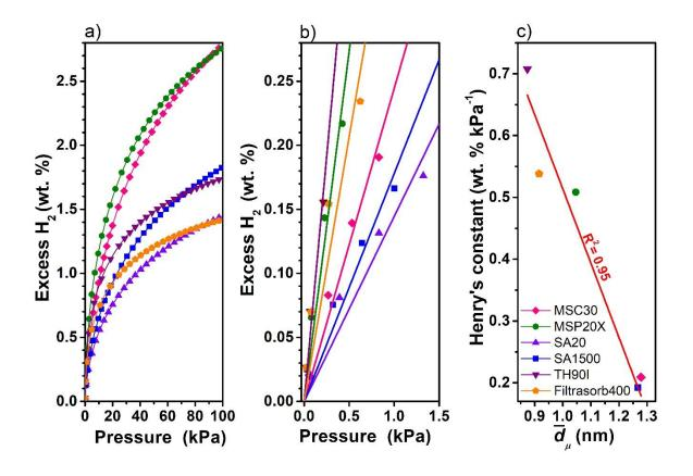
**Figure 5.** Hydrogen isotherms for the six CACs at 77 K: (a) up to 100 kPa; and (b) up to 1.5 kPa. (c) Henry's constant as a function of average micropore size. The legend in (c) also applies to (a) and (b).
