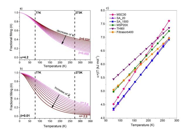
Figure 11. Effect of the parameters: (a)  $\beta$ ; and (b)  $\alpha$  on the H<sub>2</sub> adsorption capacity at  $P/P_0 = 0.02$  at different temperatures; (c) sum of enthalpy and entropy contributions as a function of temperature.
