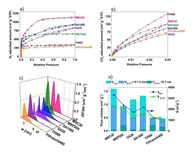
**Figure 1.** Textural characteristics of the CACs: (a)  $N_2$  adsorption-desorption isotherms at 77K; (b) CO<sub>2</sub> adsorption isotherms at 273 K; (c) Pore size distributions; (d)  $A_{BET}$ ,  $S_{NLDFT}$  and pore volumes in the ultramicropore (<0.7 nm), supermicropore (0.7-2 nm) and mesopore (2-50 nm) ranges.
