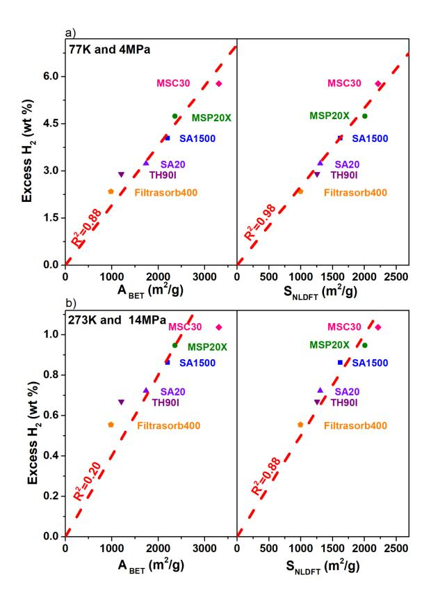
**Figure 4.** Hydrogen excess adsorbed as a function of  $A_{BET}$  or  $S_{NLDFT}$  at: (a) 77 K and 4 MPa (value for Filtrasorb400 corresponds to 3 MPa); and (b) 273K and 14 MPa. The dashed lines (---) correspond to the linear regression fit through the origin at (0,0).
