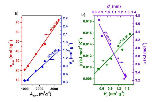
Figure 7. MDA parameters plotted as a function of several textural parameters: (a)  $V_a$  and  $n_{max}$  as a function of  $A_{BET}$ ; (b)  $\alpha$  as a function of the average micropore size, and  $\beta$  as a function of the total pore volume.
