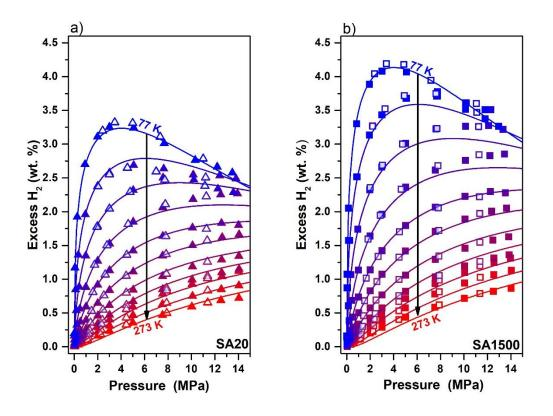
**Figure 6.** Hydrogen isotherms on: (a) SA20; and (b) SA1500, and their fitting with the MDA equation at 77, 93, 113, 133, 153, 173, 193, 213, 233, 253 and 273 K. Full and empty symbols indicate adsorption and desorption data, respectively.
