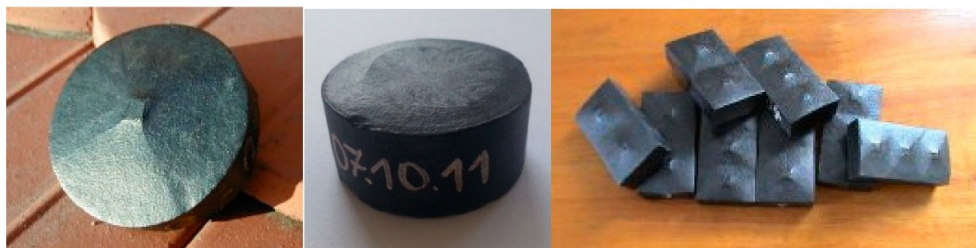
Figure 1. Mono crystal high-temperature superconducting (HTS) bulks from ATZ company.
