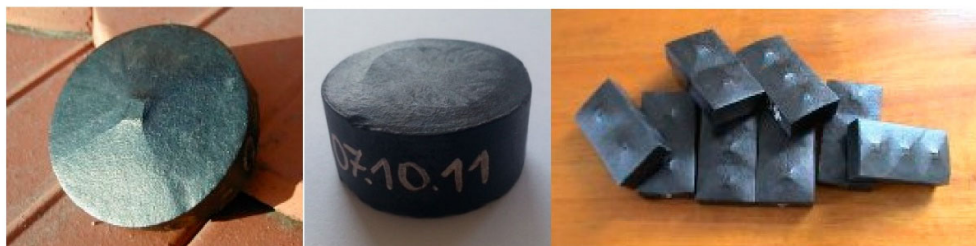
Figure 1. Mono crystal high-temperature superconducting (HTS) bulks from ATZ company.
