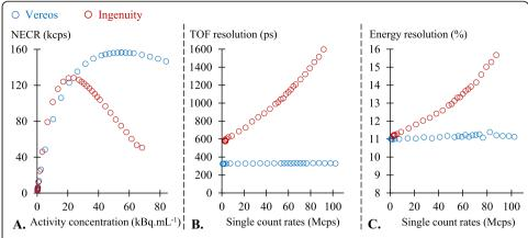
**Fig. 1** Results obtained from the NEMA count-rate test for the Ingenuity (red) and the Vereos (blue) cameras, with the relationships between noise equivalent count rates and activity concentration (NECR) (a) and with the relationships between TOF (b) or energy (c) resolutions and single-count rates
