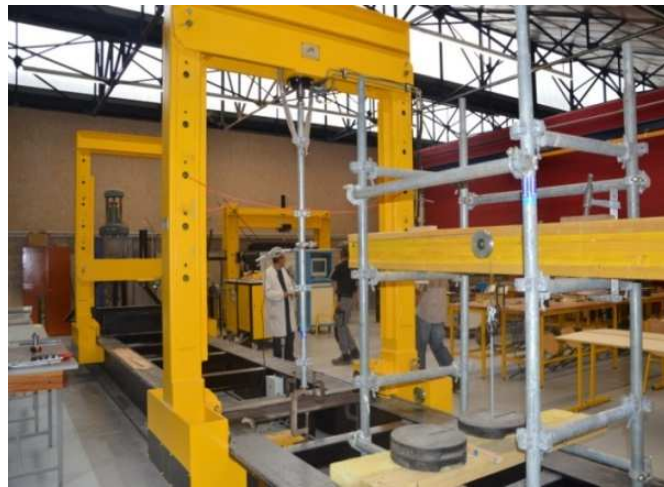
Figure 2 Simply supported members test device
