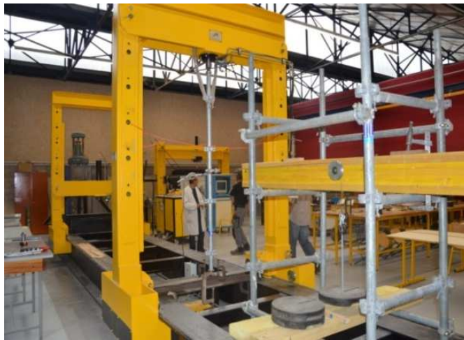
Figure 2 Simply supported members test device
