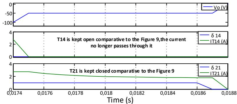
Figure 18. Voltage  $V_o$ , currents  $IT_{21}$  and  $IT_{14}$ , and switching patterns  $\delta_{21}$  and  $\delta_{14}$  (Zoom 4).
