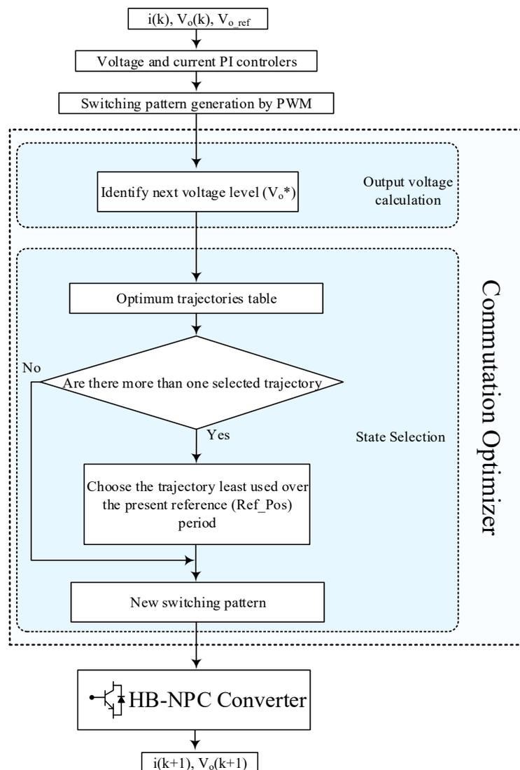
Figure 13. The final algorithm for OPTimized (OPT)-PWM.
