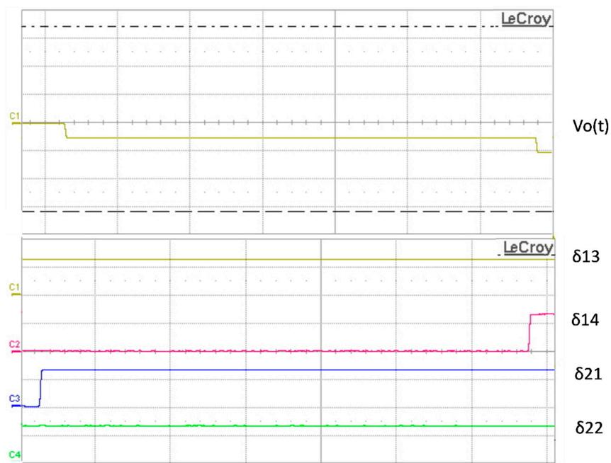
Figure 25. Output voltage  $V_o(t)$  and switching patterns sent to T13, T14, T21, and T22 (ZOOM 2 of Figure 23).
