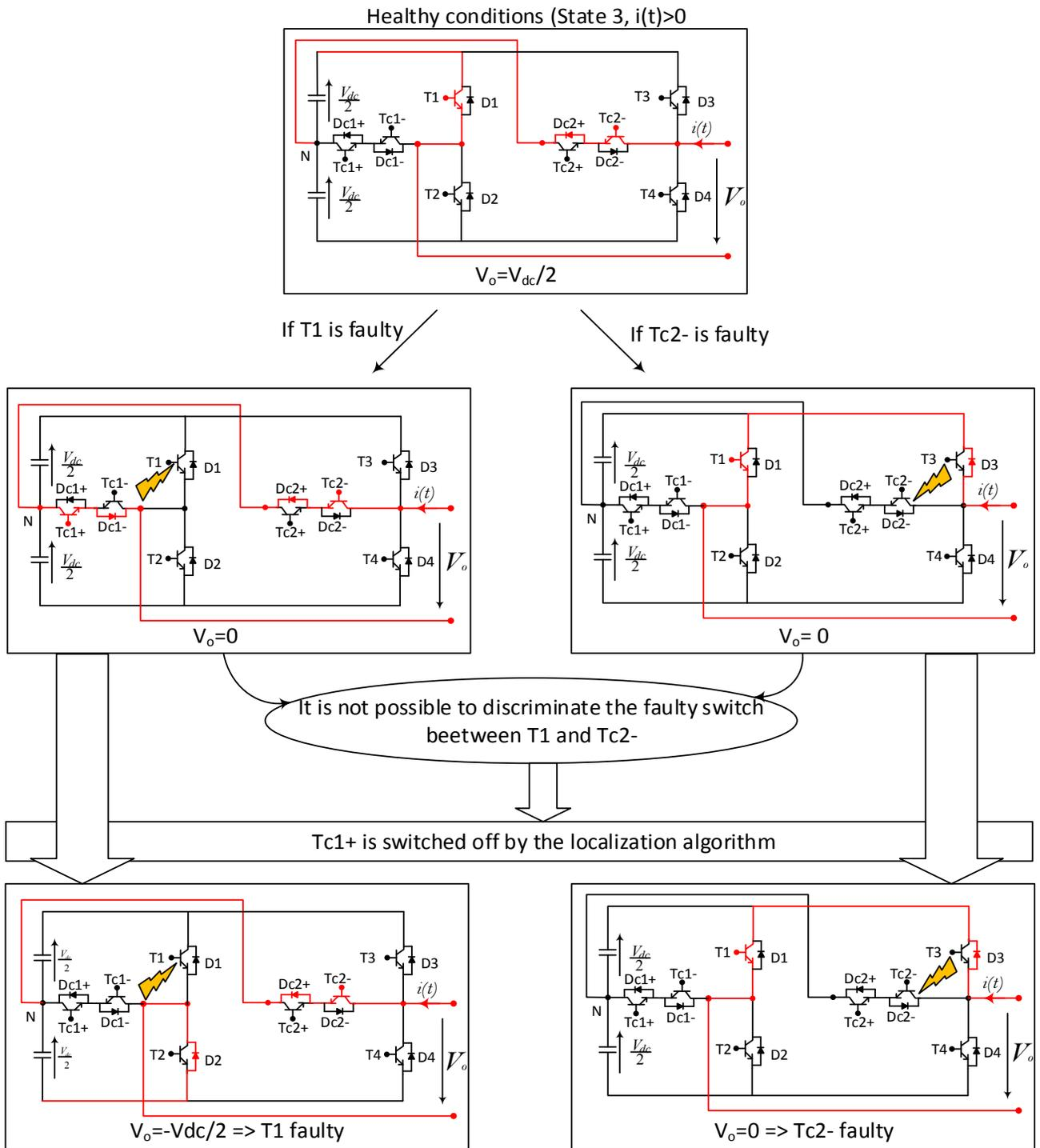
Fig 5. Open switch fault diagnosis in State 3.
