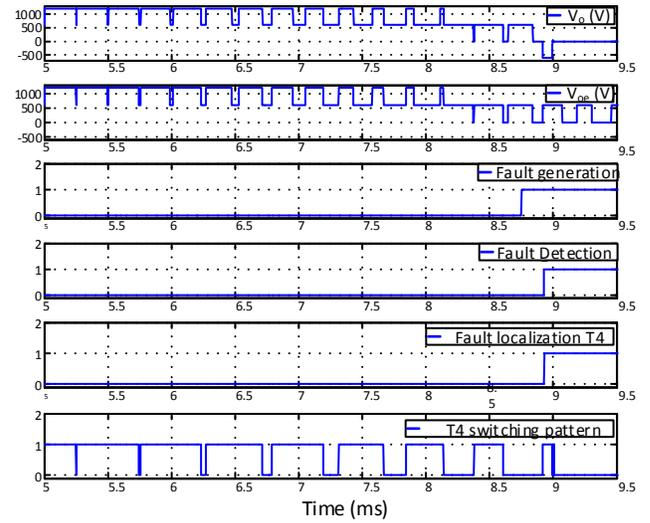
Fig. 9 Simulation results when T4 is faulty (OCF).
