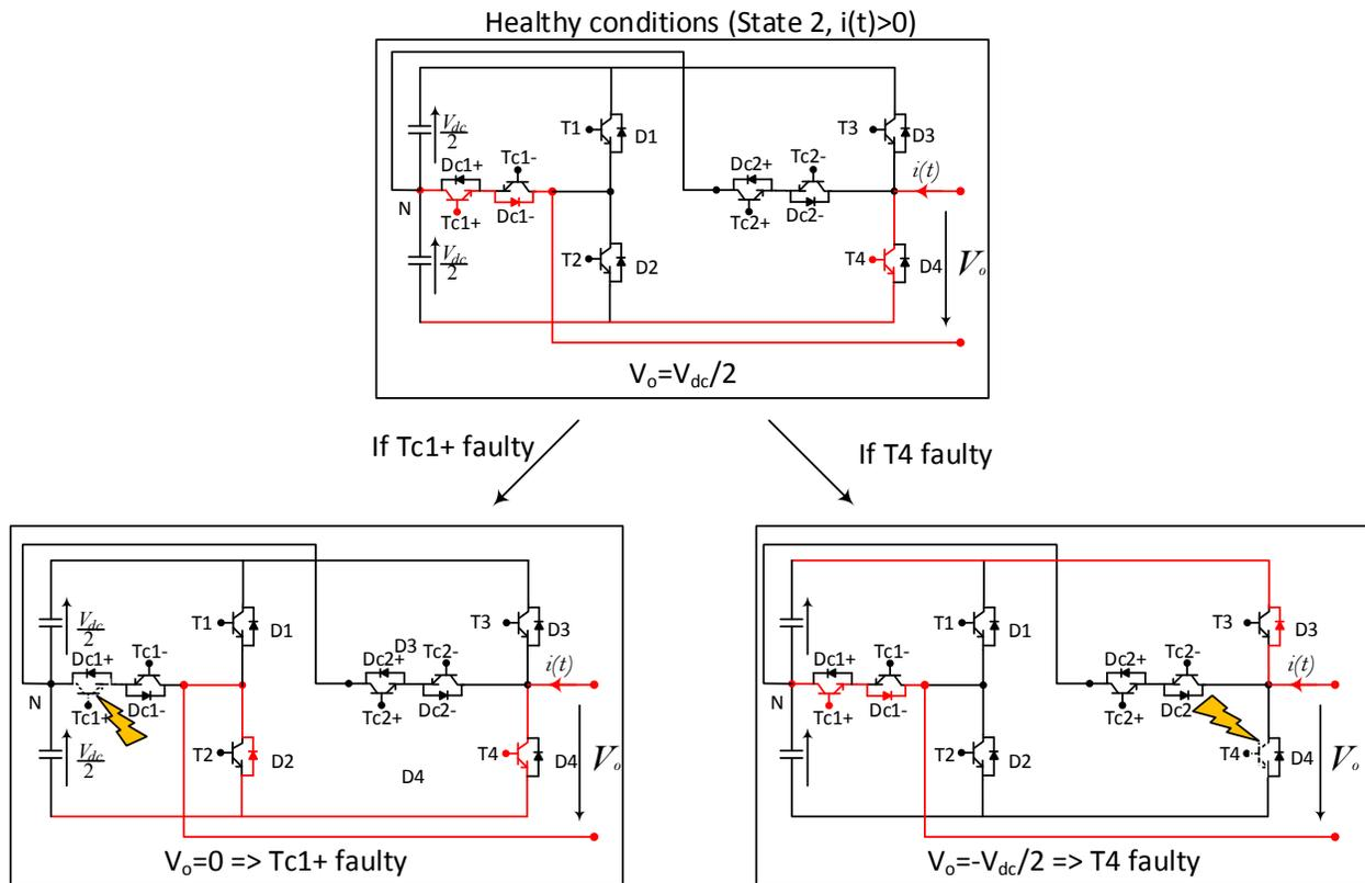
Fig. 4. Open switch fault diagnosis in State 2 ( $i(t)>0$ ).
