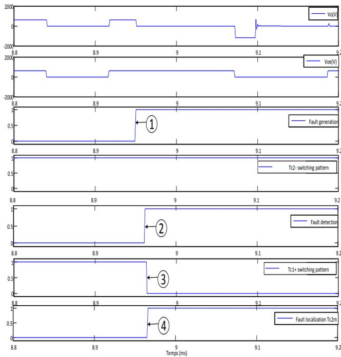
Fig. 14 : Zoomed Simulation results when Tc2- is faulty.
