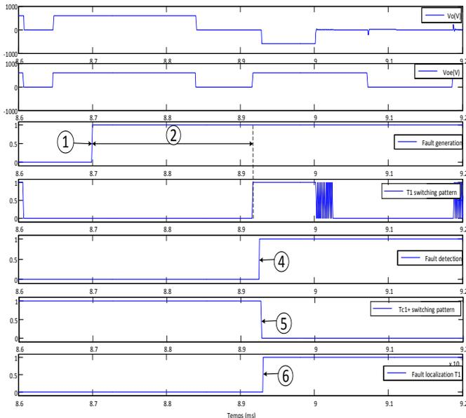
Fig. 12: Zoomed Simulation results when T1 is faulty.
