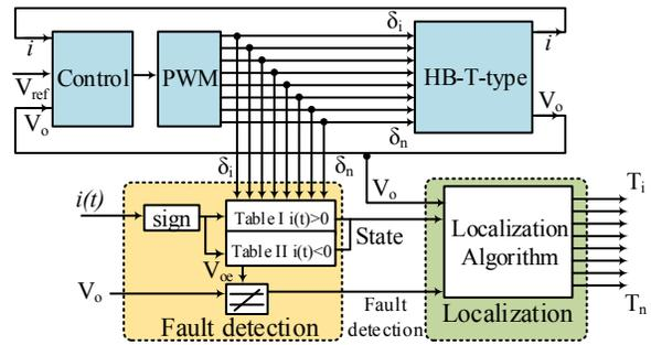
Fig. 3 Fault diagnosis principle for a T-type converter
