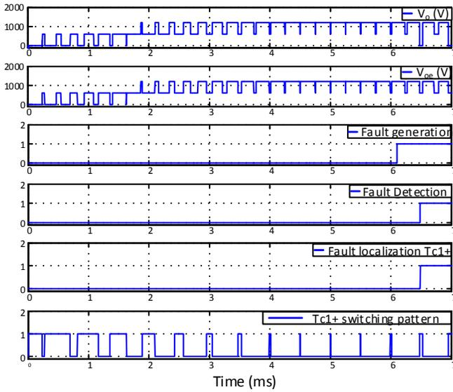
Fig. 7 Simulation results when Tc1+ is faulty (OCF).
