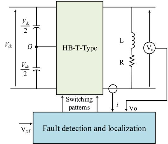
Fig. 6 HB-T-Type connected to a (R, L) load.
