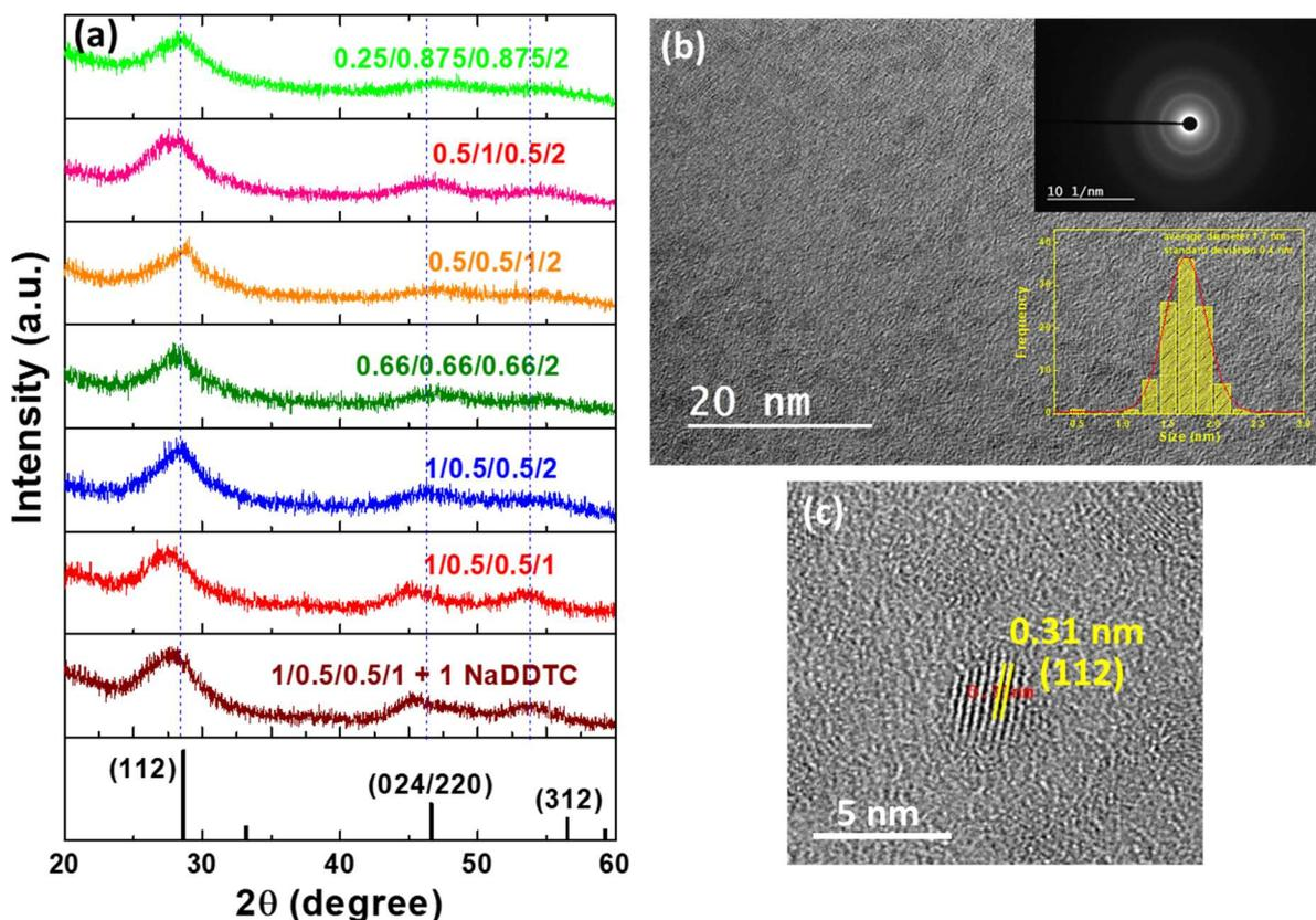
**Fig. 4.** (a) XRD patterns of AIGZS QDs, (b) TEM image and (c) HR-TEM image of AIGZS QDs prepared with a Ag/In/Ga/Zn ratio of 1/0.5/0.5/2. The insets of (b) are the SAED pattern and the size distribution.
