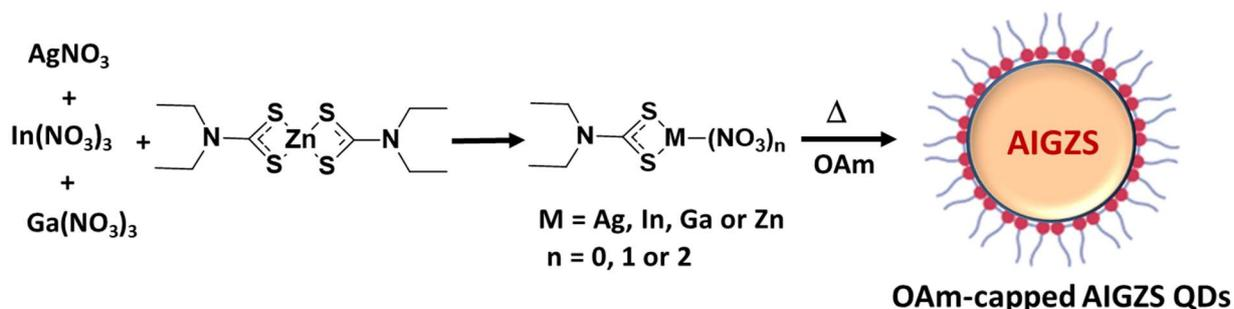
**Scheme 1.** Schematic representation of AIGZS QDs synthesis.
