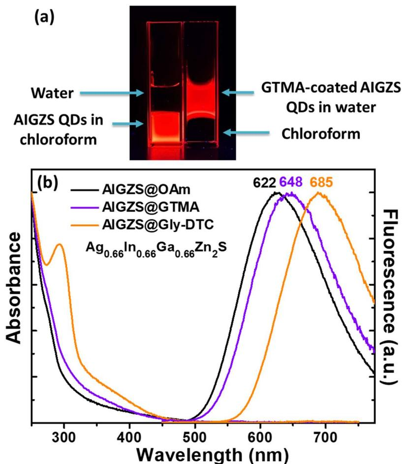
**Fig. 6.** (a) Digital photograph taken under UV light illumination of dispersions of AIGZS QDs before and after the ligand exchange with GTMA. (b) UV-visible and normalized PL emission spectra of AIGZS QDs capped with OAm and after their transfer into water using GTMA and Gly-DDTC ligands.
