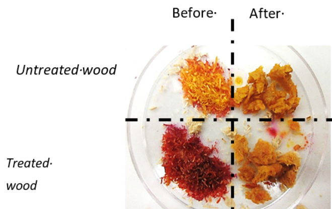
Figure 5. Colorimetric copper with (Pyridyl-2-azo)-1-naphthol-2 (PAN) in milled wood sample before or after bioprocessing treatment. The loss of wood stain shows the decontamination of copper from wood by microorganisms.
