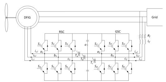
Fig. 2. Studied fault-tolerant system.
