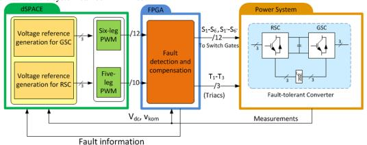
Fig.7. Proposed reconfigurable control.
