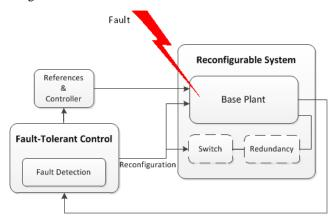
Fig. 1. General presentation of a fault tolerant system.
