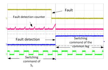
Fig. 26. Fault detection for S<sub>3</sub> (top to bottom): Fault, Fault detection counter, Fault detection, S<sub>3</sub>/shared leg's switching command – Time scale: 100µs/div.
