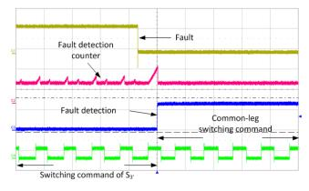
Fig.21. Fault detection for an open-circuit switch fault in  $S_3$ ' from (top to bottom): Fault signal, Fault detection counter, Fault detection,  $S_3$ '/shared leg's switching command- Time scale:  $100\mu s$ /div.
