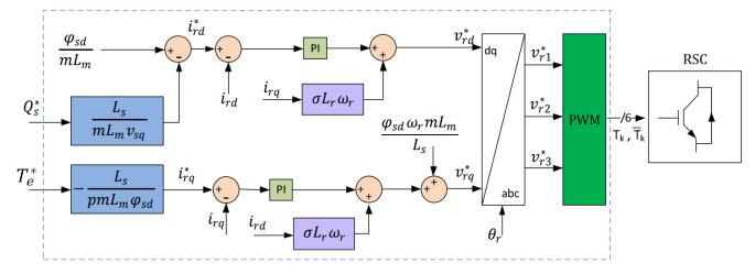
Fig. 5. Block diagram of the control of rotor voltages and currents.
