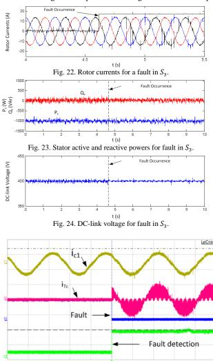
Fig. 25. Fault detection for  $S_3$  (top to bottom): Faulty leg's current  $i_{c1}$ , TRIAC's current  $i_{Tc}$  (20 A/div), Fault signal, Fault detection – Time scale: 100ms/div.
