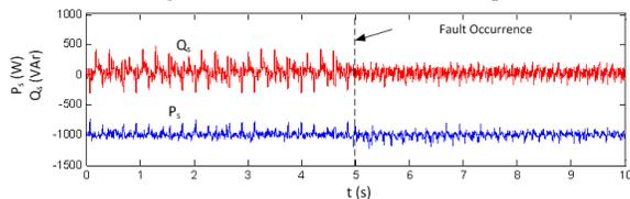
18 Fig. 18. Stator active and reactive powers for a fault in  $S_3'$ .
