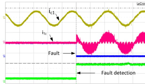
Fig. 25. Fault detection for  $S_3$  (top to bottom): Faulty leg's current  $i_{c1}$ , TRIAC's current  $i_{Tc}$  ( $20\ \text{A}/\text{div}$ ), Fault signal, Fault detection – Time scale:  $100\text{ms}/\text{div}$ .
