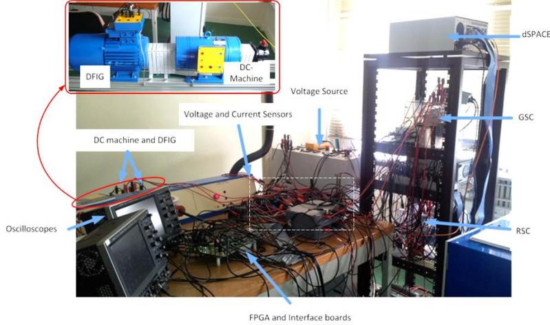
Fig. 15. Experimental set-up
