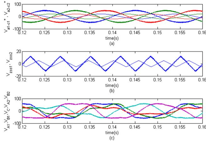
7 Fig. 4. Example of five-leg reference generation; (a): two sets of three-phase references; (b): two ZSSs; (c): resulted five-leg references.
