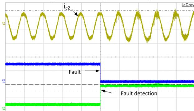
22 Fig. 20. Fault detection for an open-circuit switch fault in  $S_3'$  (from top to bottom):  $i_{c2}$  (5 A/div), Fault signal, Fault detection – Time scale: 20ms/div.
