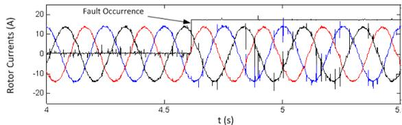
Fig. 22. Rotor currents for a fault in  $S_3$ .
