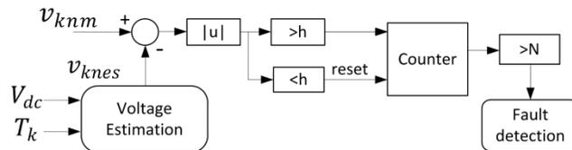
38 Fig.8. Fault detection scheme.
