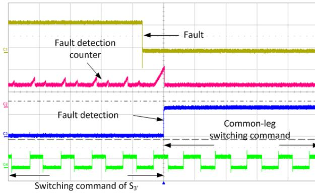
Fig.21. Fault detection for an open-circuit switch fault in  $S_3'$  from (top to bottom): Fault signal, Fault detection counter, Fault detection,  $S_3'$ /shared leg's switching command- Time scale:  $100\mu\text{s}/\text{div}$ .
