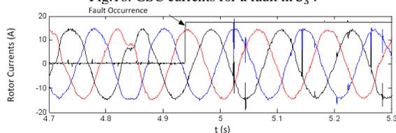
16 Fig. 17. Rotor currents for a fault in  $S_3'$ .
