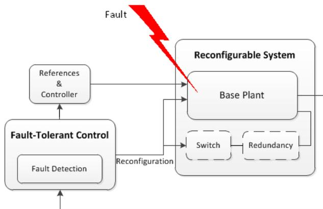
29 Fig. 1. General presentation of a fault tolerant system.
