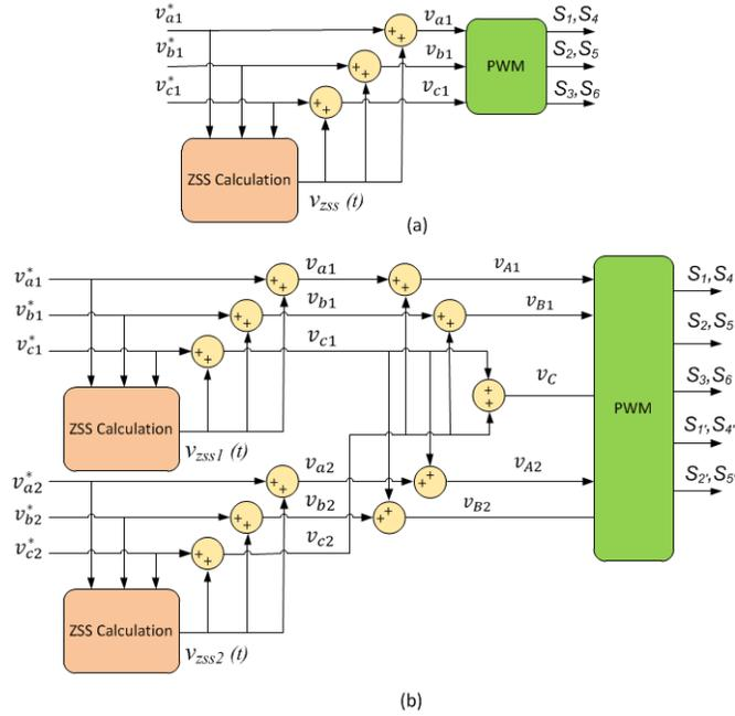
5 Fig. 3. Principle of PWM control module: (a) for a three-phase converter; (b) for a 5-leg converter when the legs “c” are shared.
