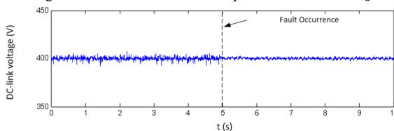
20 Fig. 19. DC-link voltage for a fault in  $S_3'$ .
