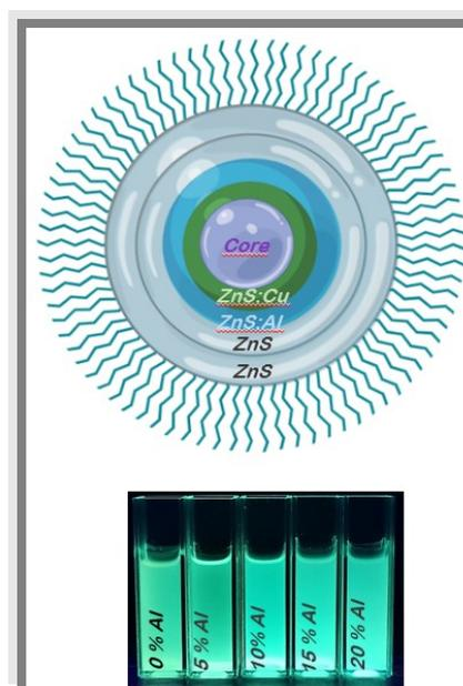
**Figure 1:** Schematic illustration of the structure of Cu,Al:ZnSeS/ZnS QDs and digital photograph taken under UV light illumination of the dots when varying the Al<sup>3+</sup> dopant percentage.
