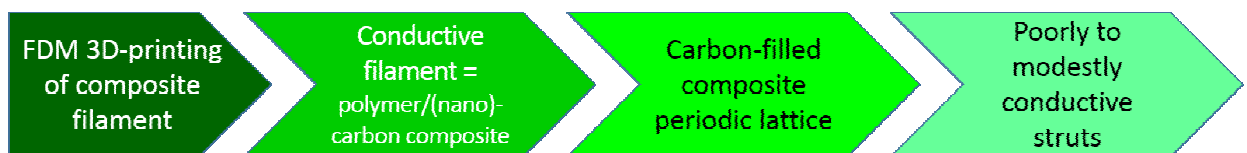
Figure 1. Schematic representation of two basic approaches for 3D-printing electrically conductive, carbon-based periodic lattices.
