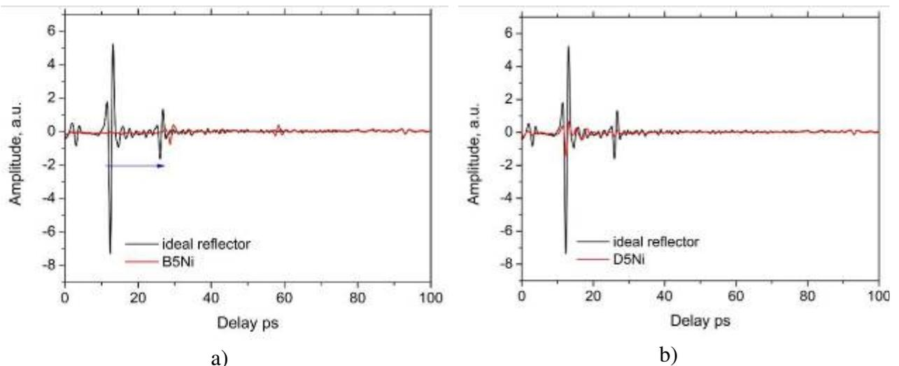
**Figure 10.** Impulse of the reflected THz signal for the case of an ideal reflector (black line) and for 3D glassy carbon periodic structures based on: (a) large (B5Ni); and (b) small (D5Ni4) Kelvin cells (the arrow indicates the time delay).
