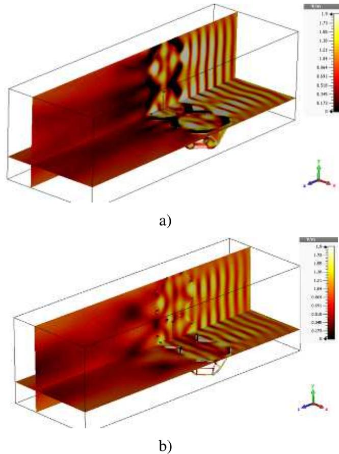
**Figure 6.** Calculated amplitude of the electric field vector for carbon-based Kelvin cells having two strut thicknesses: (a)  $d = 0.5$  mm and (b)  $d = 0.1$  mm. Numerical simulations were performed with a backbone dc conductivity of  $20\,000\text{ S m}^{-1}$  and a strut length of 1 mm.
