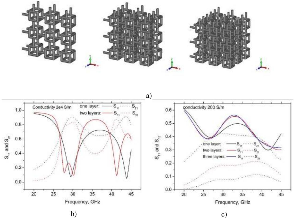
**Figure 7.** Frequency dependence of  $S_{11}$  and  $S_{21}$  parameters for a 3D structure based on one, two, or three layers of Gibson-Ashby cells as pictured in (a), and for two different values of backbone dc conductivity: (b)  $20\,000\text{ S}\cdot\text{m}^{-1}$ ; and (c)  $200\text{ S}\cdot\text{m}^{-1}$ . The following geometric parameters were used in the calculation:  $l = 3\text{ mm}$ , and  $d = 0.83\text{ mm}$ .
