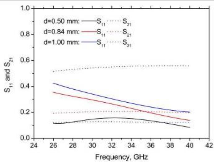
**Figure 5.**  $S$ -parameters of two layers of Gibson-Ashby cells having the three different strut thicknesses ( $d$ ) indicated on the plot, as a function of frequency. In the numerical calculation, the following parameters were used: backbone dc conductivity  $10 \text{ S m}^{-1}$ ,  $L = 2.4 \text{ mm}$ , and  $\varepsilon = 1$ .
