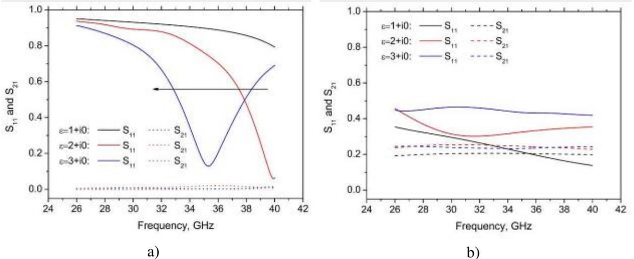
**Figure 3.** Frequency dependence of the  $S$ -parameters for one layer of Gibson-Ashby cells such that  $L = 2.4$  mm and  $a = 0.84$  mm, for different relative permittivity values  $\epsilon$  of the impregnation medium and two values of dc electrical conductivity of the carbon backbone: (a)  $2\,000\text{ S m}^{-1}$ ; and (b)  $10\text{ S m}^{-1}$ .
