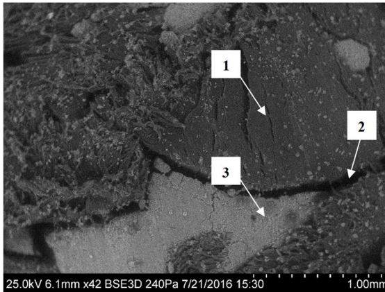
Fig. 5. SEM image of hemp concrete (1 mm): (1) Hemp shiv (2) Porosity (3) Binder
