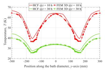
Fig. 3. Comparison of the nitrogen temperature distribution over the bath diameter after 10h and 30h of cooling.
