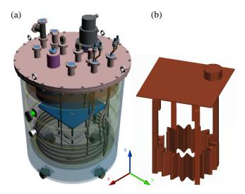
Fig. 1. Cryostat manufactured by Cryo Diffusion (a), and the heat exchanger designed to solidify nitrogen by using a Sumitomo CH-110 crycooler (b).
