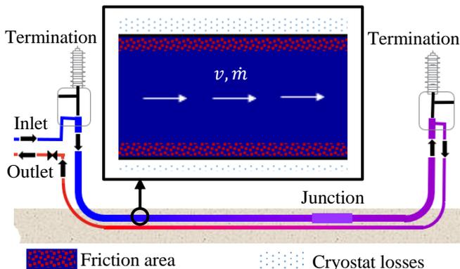
Fig. 1. Schematic illustration of a cryogenic line with Separate Pipes.
