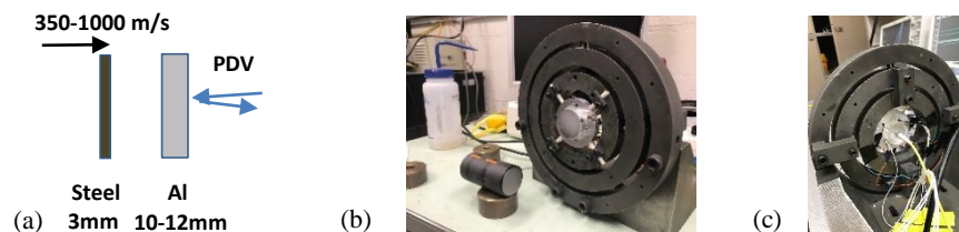
FIGURE 1. Plate impact experimental set up: (a) schematic, (b) target assembly on alignment gimbal and (c) PDV mounted on the back side.
