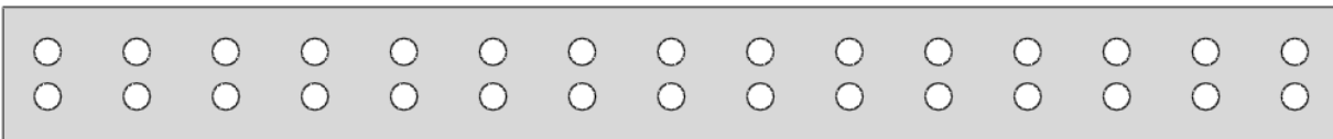
Fig. 4: 2D beam with a regular distribution of periodic holes as a microstructure
