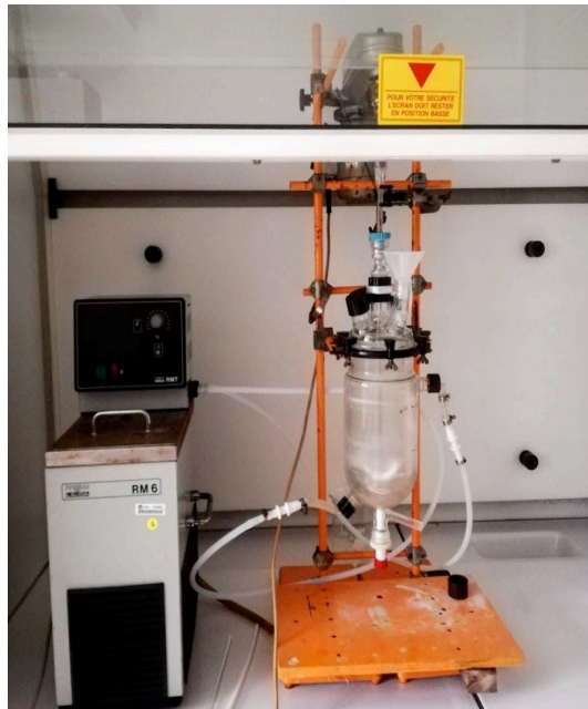
518 519 Figure 2: Setup for leaching experiments.
