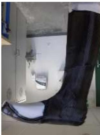
Photo 5: Stratification du carbone
