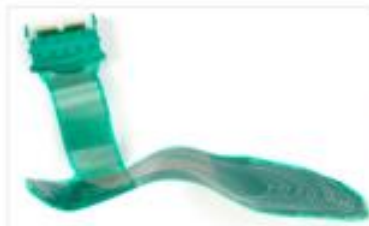
Flexible, thin in-shoe sensors give information about what's occurring inside the shoe.
