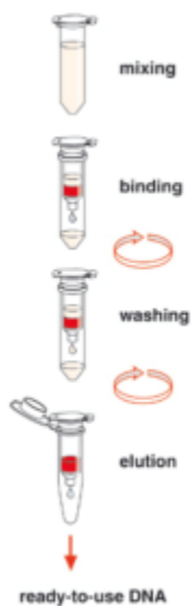
Figure 13: Principe d'utilisation du kit NucleoSpin plasma XS (BIOKE)
