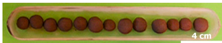
Figure 9. Optical image of pellets (35% hematite + 35% W-PVC + 30% clay) treated at 300 °C for 30 min.
