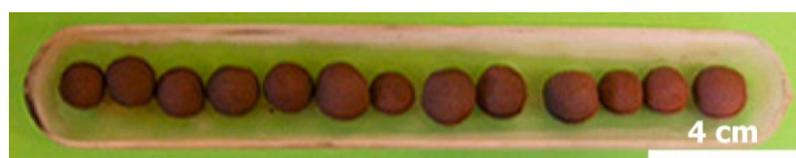
Figure 9. Optical image of pellets (35% hematite + 35% W-PVC + 30% clay) treated at 300 °C for 30 min.
