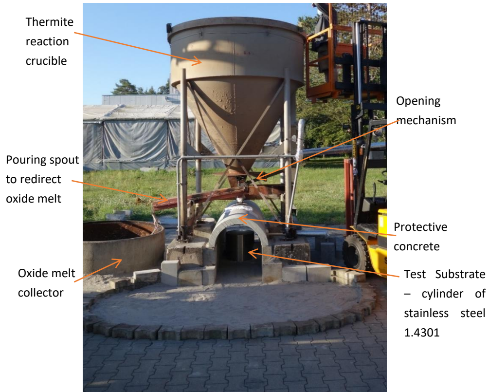
Fig. 7: Picture of JIMEC 2 test set-up
