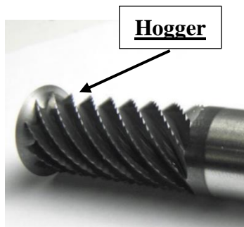
Figure 2. Milling cutter used for Nomex® honeycomb core "CZ10".
