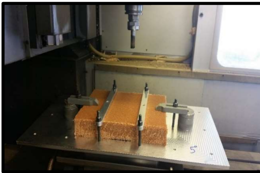
Figure 7. Experimental test setup on the three-axis vertical machining center. (a)- Instrumentation and acquisition system. The characteristics of the machine-tool are: maximum spindle speed of 24000 rpm, power spindle motor of 30 KW, maximum cutting feed rate of 20 m/min and a worktable area of 800 x 600 mm 2 . (b)- Workpiece Fixing and cutting directions.
