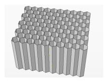
Figure 1: Diagram of the honeycomb structure.
