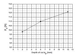
Figure 12: Evolutions of thrust forces F<sub>z</sub>
