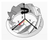
Figure 3: Cutting conditions assigned to the cutting tool, N is the speed of rotation, f is the feed rate.
