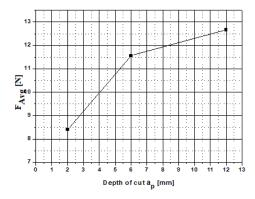
Figure 9 : Evolutions of cutting forces  $F_{\mbox{\scriptsize Avg}}$
