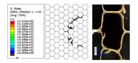
Figure 14: Comparison between the surface quality obtained during the machining of the Nomex honeycomb (Jaafar 2018) and the surface quality resulting from the digital simulation, the cutting conditions are:  $f=200\ \text{mm}\ /$  min and  $N=2000\ \text{rpm}$ .
