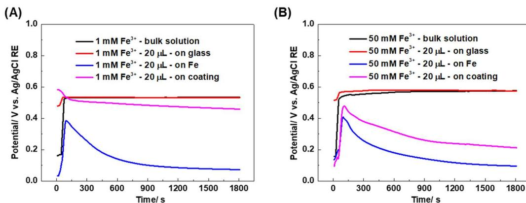
**Fig. 6.** OCP measurements by integrated probe in Fe<sup>3+</sup> bulk solution, 20 μL Fe<sup>3+</sup> droplet on insulating glass, bare and silane-treated Fe substrates. (A): 1 mM Fe<sup>3+</sup>, (B): 50 mM Fe<sup>3+</sup>.
