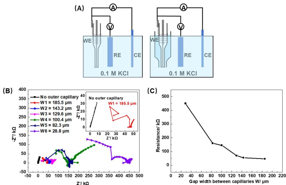
**Fig. 3.** (A) Scheme of EIS measurement; (B) Nyquist plots of Ag/AgCl wire of the integrated probe in 0.1 M KCl solution with different gap width (W) between inner electrodes and outer capillaries; (C) Ion transfer resistance of integrated probes with different gap width.
