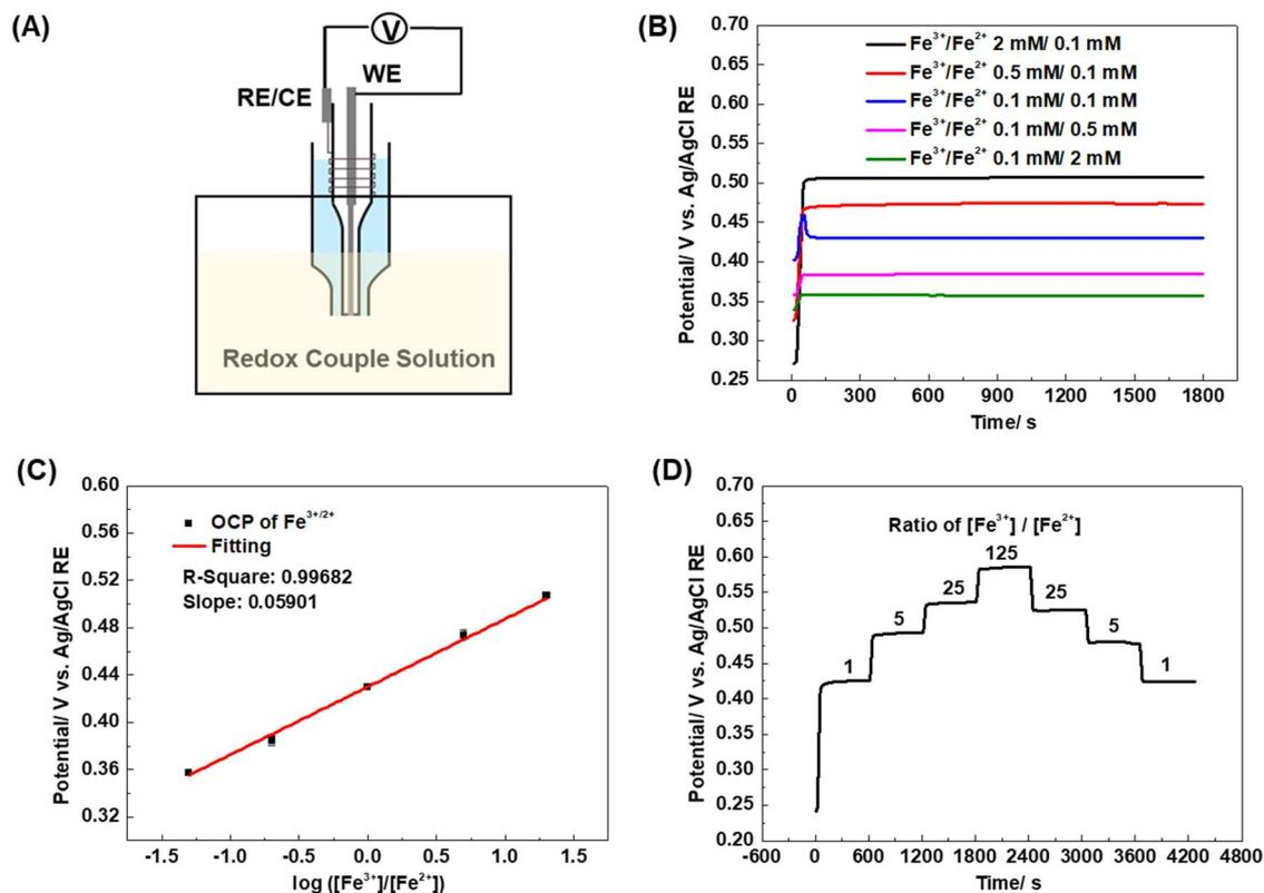
**Fig. 4.** (A) Scheme of potentiometric measurements of the integrated probe in bulk solutions; (B) Potential variation in  $\text{Fe}^{3+}/\text{Fe}^{2+}$  redox solutions with different concentration ratio; (C) Potential versus  $\log([\text{Fe}^{3+}]/[\text{Fe}^{2+}])$ ; (D) Potential steps following the variation of  $[\text{Fe}^{3+}]/[\text{Fe}^{2+}]$  ratio in the solution.
