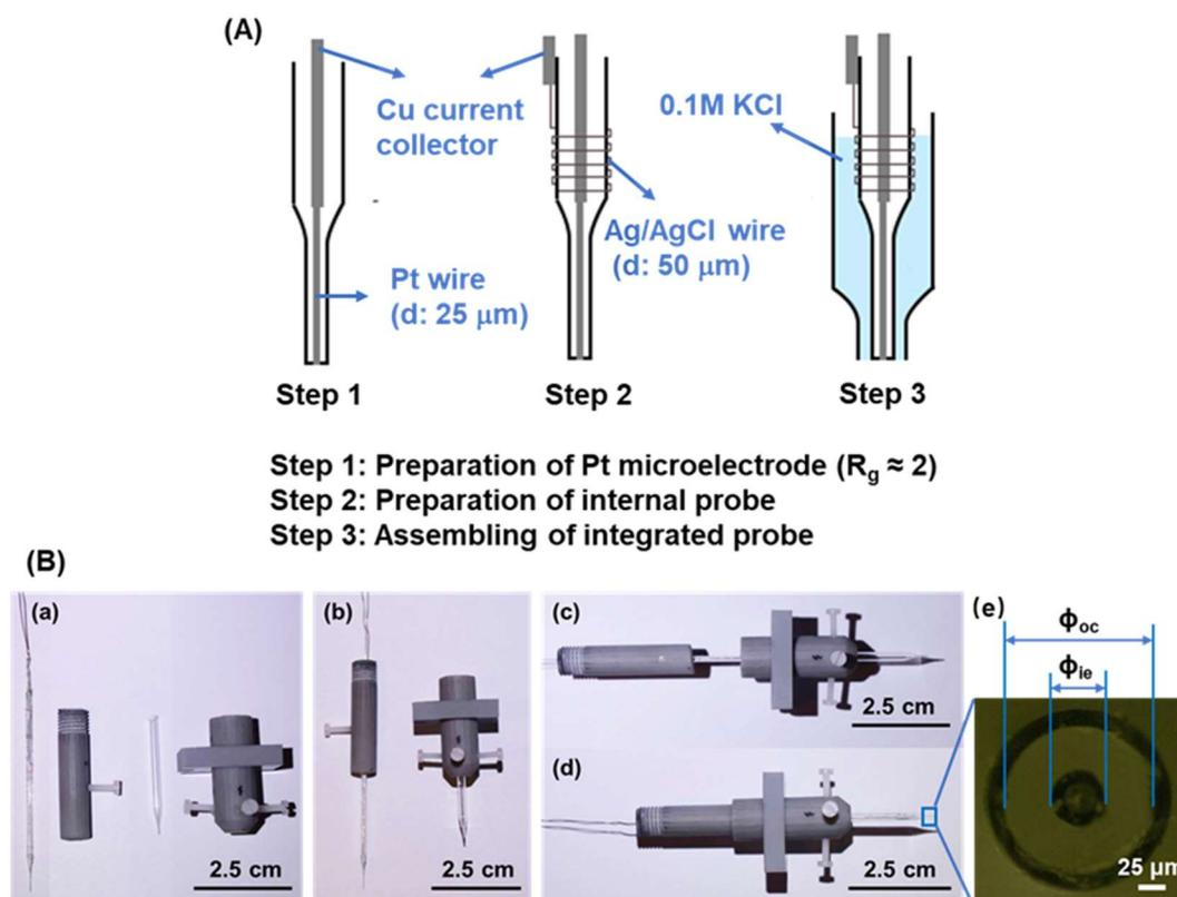
**Fig. 1.** (A) Scheme of the fabrication of integrated probe. (B) (a-d) Photographs illustrating different steps of the fabrication, (e) tip of the integrated probe, gap width ( $W$ ) = inner diameter of outer capillary ( $\phi_{oc}$ ) – outer diameter of inner electrode ( $\phi_{ie}$ ).
