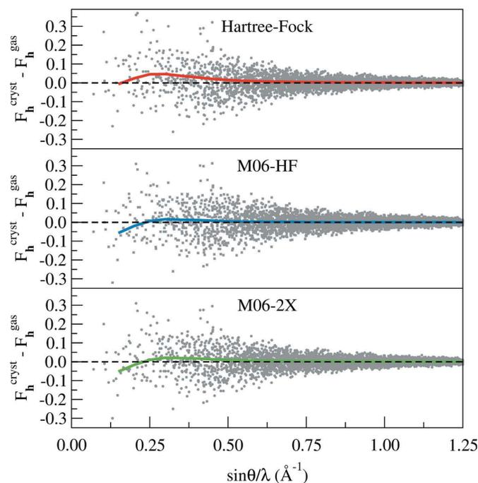
**Figure 3** Discrepancies between the standard and MOLSPLIT structure factor amplitudes ( $F_{\text{h}}^{\text{cryst}}$  and  $F_{\text{h}}^{\text{gas}}$ , respectively) at different levels of theory. The solid curves show the trends of the average discrepancy as a function of  $\sin\theta/\lambda$ .
