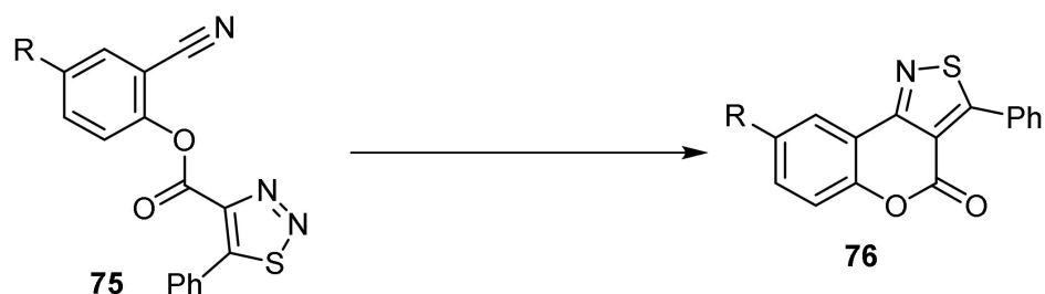
Scheme 22. Synthesis of 8-substituted-3-phenyl-4H-chromeno[4,3-c]isothiazol-4-ones 76 . Reagents and conditions. An amount of 5.0 mol% [\text{Rh}(\text{COD})\text{Cl}]_2 , 12.0 mol% DPPF, PhCl (1.0 mL), N 2 , 80 °C; R = H 90% yield; R = Me 99% yield; R = Br 90% yield.
