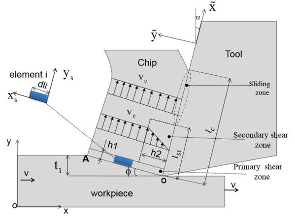
Figure 1: Illustration of an orthogonal cutting operation
