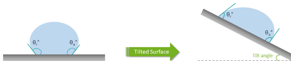
FIGURE 5 Receding and advancing contact angles determining contact angle hysteresis
