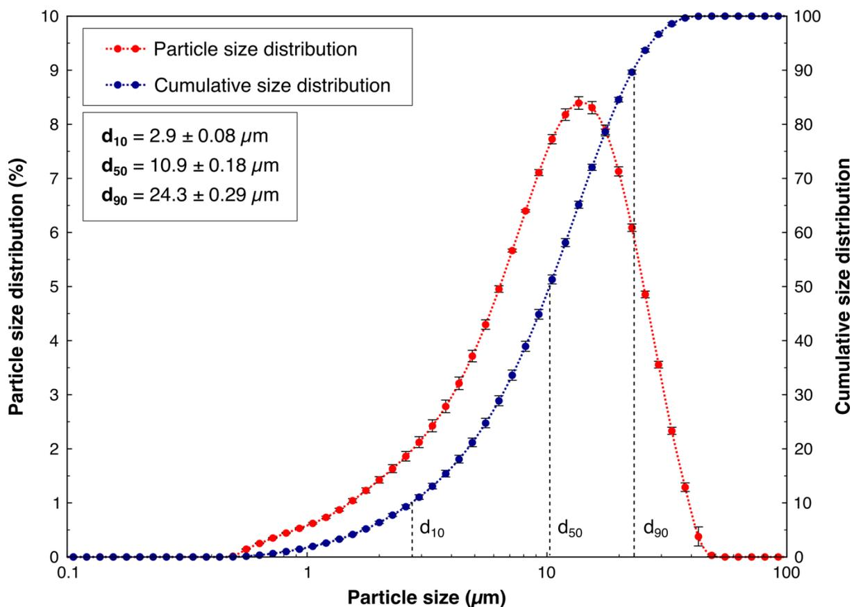
Figure 2. Particle size distribution and cumulative size distribution of scheelite used for adsorption experiments.  $d_{90}$ ,  $d_{50}$ , and  $d_{10}$  correspond to the diameters below which 90, 50 and 10% of the particles can be found, respectively.
