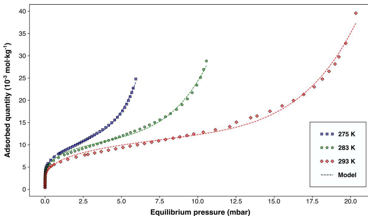
Figure 3. Adsorption isotherms of gas water on scheelite at 275, 283, and 293 K (dots) and their fits with the Dual-Site Freundlich-Langmuir model (Eq. 4, dashed lines).
