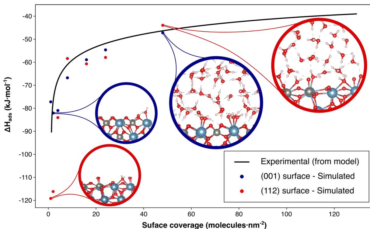
Figure 7. Adsorption energies per water molecule for the (001) and (112) scheelite surfaces when the water coverage is increased from 1 to 48 water molecules (for surfaces of around  $1 \text{ nm}^2$ , which therefore represents a coverage of 1 to  $48 \text{ nm}^{-2}$ ).
