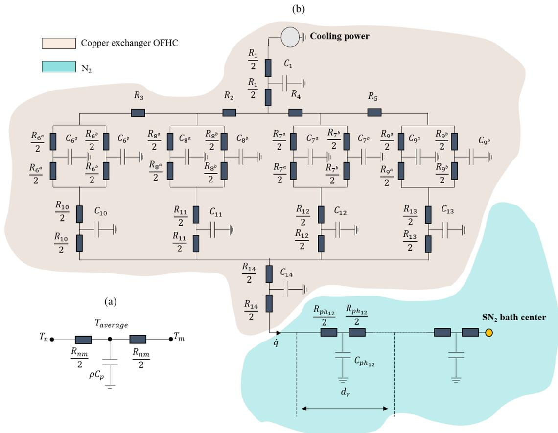
**Figure 2.** (a) Thermoelectric circuit by analogy of a single element, (b) Simplified schematic of the nodal network, the beige area represents the copper parts and the blue area represents the radial discretization in the nitrogen bath. The indexes of each resistance and thermal capacity of the copper part correspond to the numbering of the parts indicated in figure 1.
