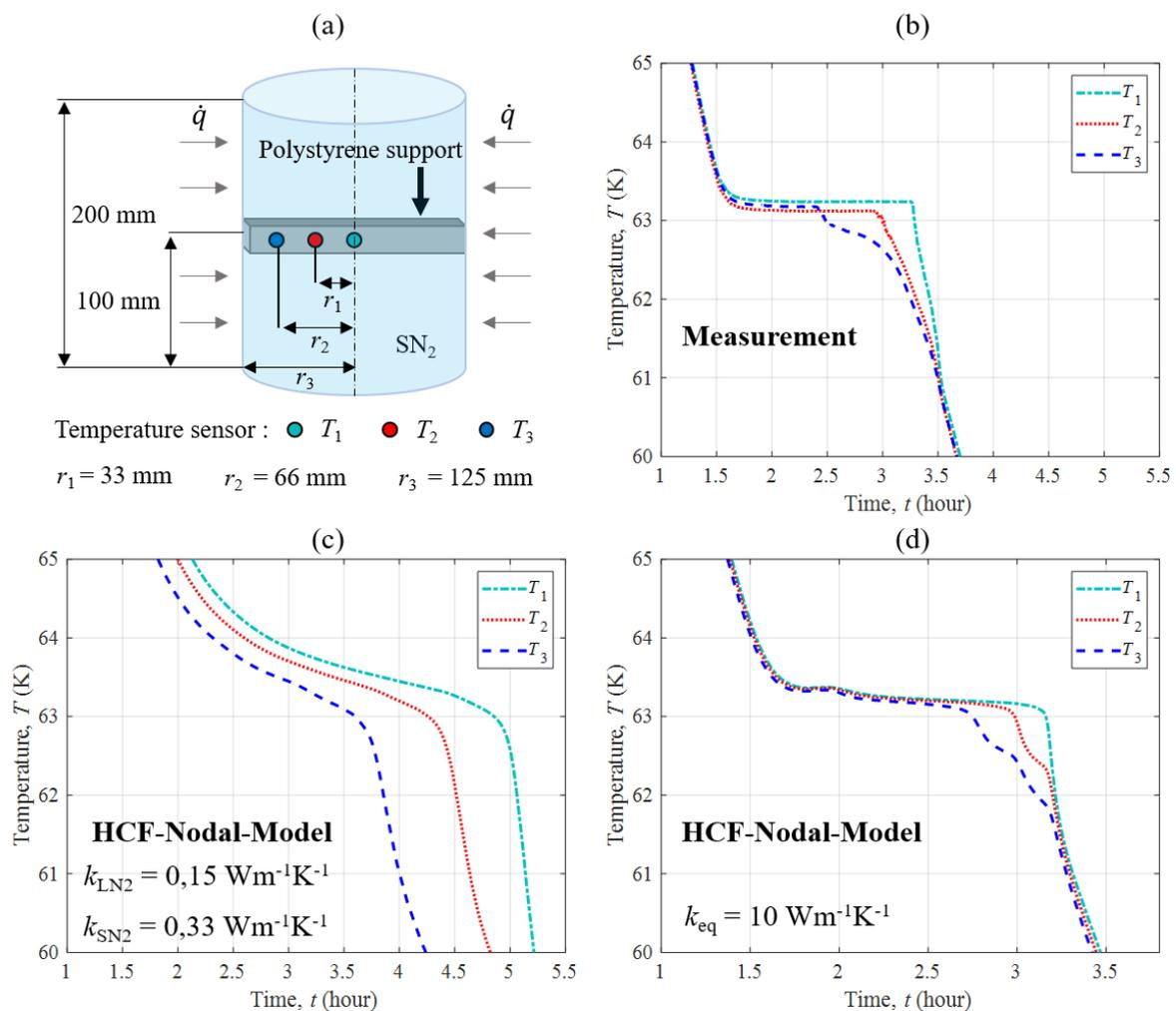
**Figure 8.** (a) Simplified diagram of the location of the temperature sensors in the nitrogen bath, (b), (c) and (d) sensor temperatures as a function of time of liquid-solid phase change for 10 L of liquid nitrogen.
