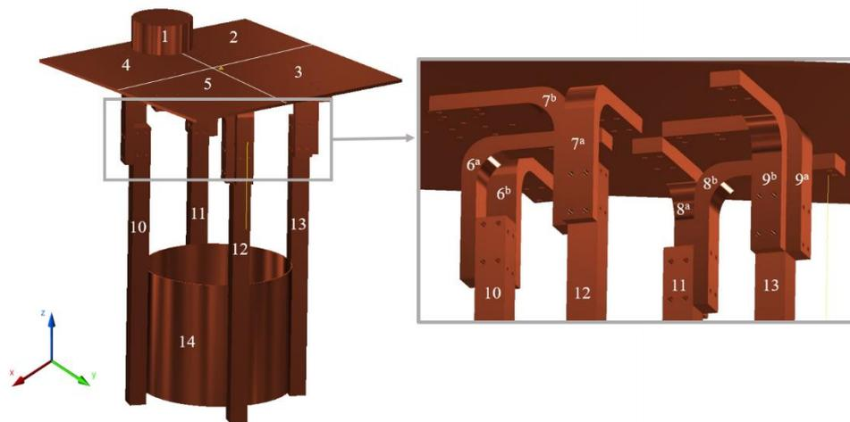
**Figure 1.** 3D view of the heat exchanger fabricated in our laboratory designed to solidify nitrogen using a Sumitomo CH-110 cryocooler and the notation of the different parts implemented in our nodal model.
