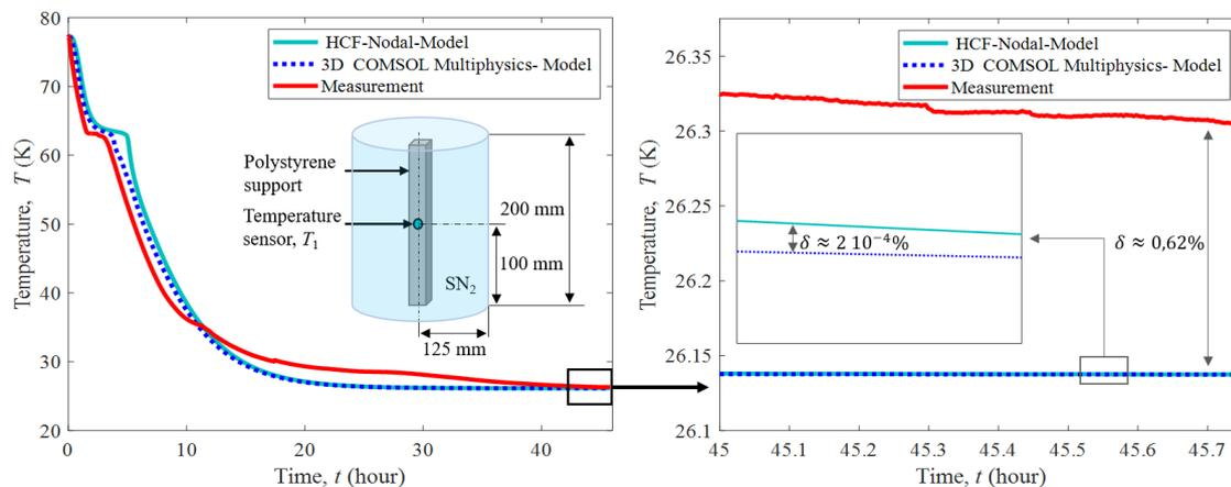
**Figure 7.** (a) Temperature at the center of the nitrogen bath as a function of time, (b) Steady state temperature in the range of 45 hours after the start of the cooling.
