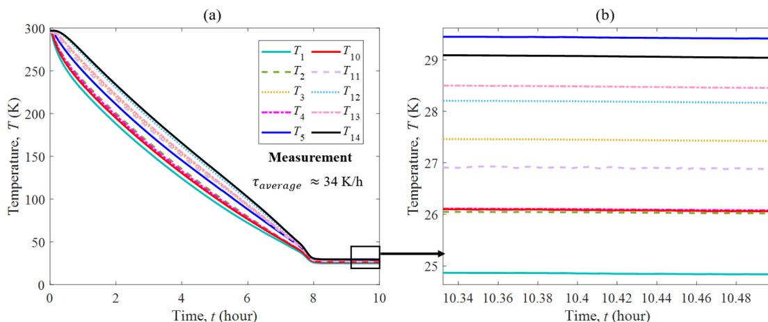
**Figure 5.** (a) A no-load test of the temperature of the different cooling system elements as a function of time, (b) Steady state temperature in the interval of 10 hours after the start of cooling. The indices of each sensor correspond to the part numbering shown in figure 1.
