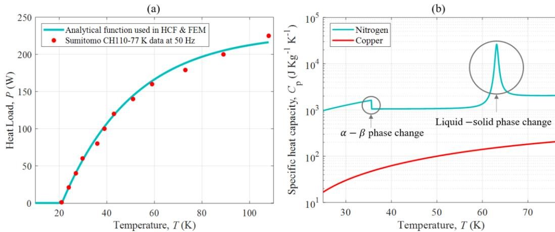
**Figure 6.** (a) Analytical formula of the cooling capacity of the Sumitomo cryocooler CH-110 77K, (b) Analytical expression of the variation of the specific heat of copper and nitrogen used in HCF-Nodal-Model and FEM.
