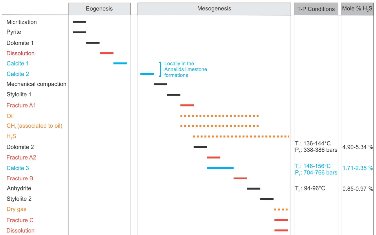
686 687 Figure 14. Paragenesis of the Lacq gas field. T t and P t correspond to the trapping T-P conditions 688 respectively as deduced from fluid modeling. T h is the homogenization temperature. The evolution of H 2 S 689 mole % is also added.
