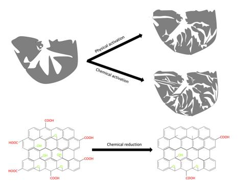
**Figure 7.** Mechanism of chemical and physical activation approaches in GO; top: modification of pore structure of GO by activation; bottom: modification of the functional groups on GO surface by activation.
