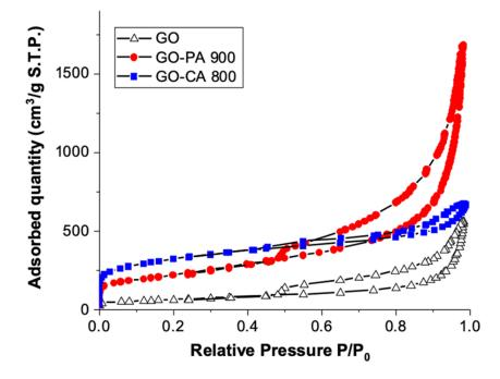
Figure 5. N<sub>2</sub> adsorption-desorption isotherms of the pristine GO, GO-PA 900 and GO-CA 800.
