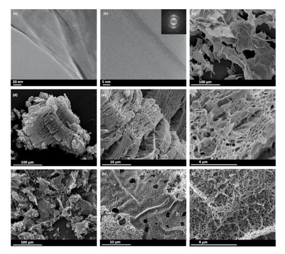
**Figure 4.** TEM images of GO (**a**) low-magnification (**b**) high-magnification, insert: corresponding FFT; (**c**) SEM image of GO; SEM images of GO-PA 900 at (**d**) low-magnification (**e-f**) high-magnification; SEM image of GO-CA 800 (**g**) low-magnification (**h-i**) high-magnification.
