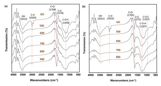
Figure 2. FTIR spectra of (a) physical activation and (b) chemical activation of GO at different temperatures.
