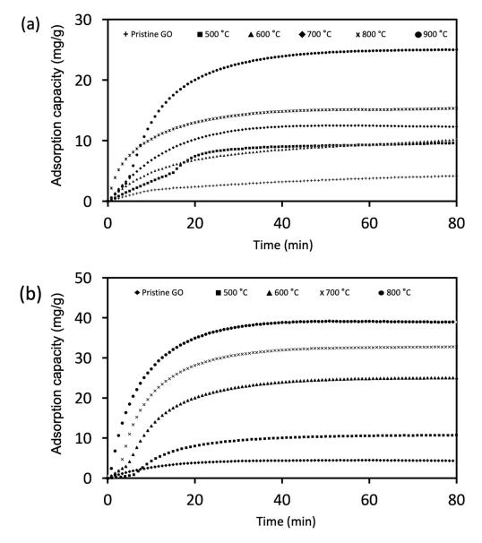
Figure 3. CO<sub>2</sub> adsorption isotherms of GO after (a) physical activation and (b) chemical activation at different temperatures.
