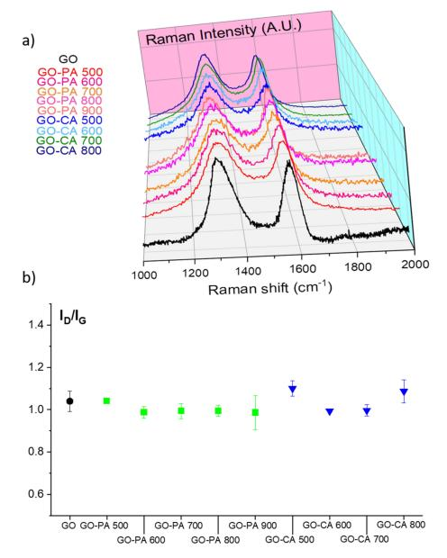
**Figure 1.** (a) Raman spectra and (b) corresponding  $I_D/I_G$  of pristine GO and the activation GO by both the chemical and the physical activation methods.
