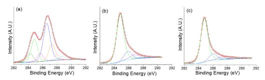
Figure 6. C 1s XPS spectra for (a) GO (b) GO-PA 900 and (c) GO-CA 800.
