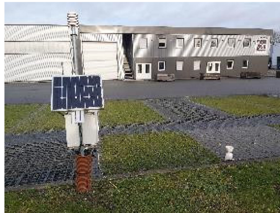
Figure 5. Data acquisition facility: outdoor temperature and relative humidity probe (CS215) on the left, rain gauge on the right (Kalyx-RG).
