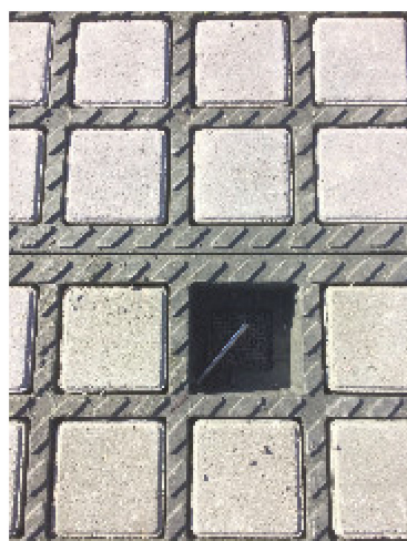
Figure 4. Example of sensor position at a depth of 3 cm in concrete paving stones (CS107). The sensor was placed inside a paving stone.
