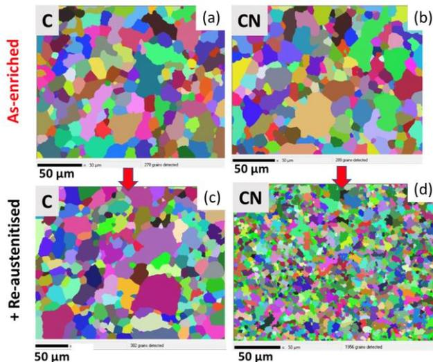
Figure 2: Evolution of the parent austenite grains upon reconstruction from EBSD data for the C, N and C+N samples in the as enriched state and upon re-austenitizing (the  $\gamma$  grains – including twins – are random colored)
