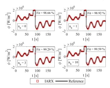
Figure 11: IARX results with the first validation case for different numbers of past exogenous parameters.
