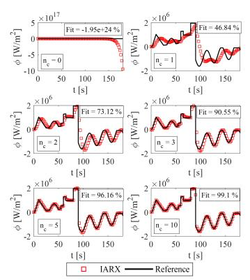
Figure 10: IARX results with the first validation case for different numbers of future exogenous parameters.
