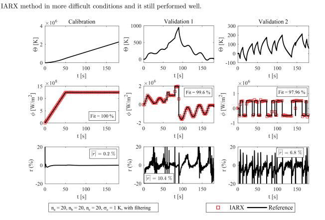
Figure 9: IARX calibration and validation with noisy temperature outputs and with filtering.
