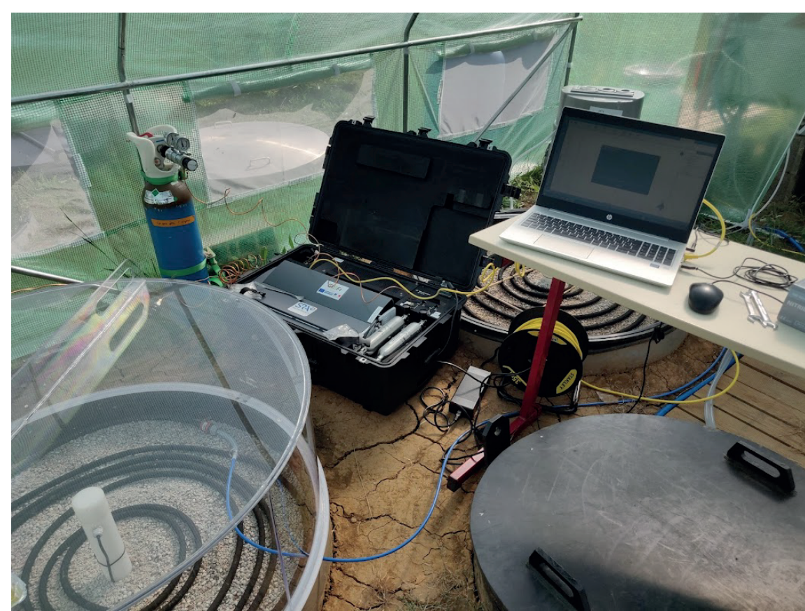
Gas collection chambers and μGC
