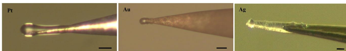
Fig. S2. Examples of sharpened hydrogel fabricated by “electrodeposition + pulling” on sharpened Pt, Au and Ag wires. Scale bar 25 \mu\text{m} .
