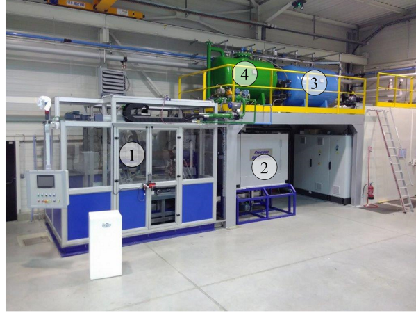
Figure 2: Photograph of the large-scale cooling experimental bench: 1) cooling chamber; 2) furnace; 3) compressed air tank; 4) pre-heated water tank.
