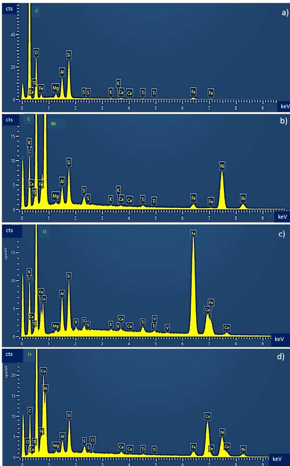
**Figure S 4:** EDS analysis of a) PGR, and the prepared electrocatalysts: b) NiO/PGR, c) Co<sub>3</sub>O<sub>4</sub>/PGR and d) NiCo<sub>2</sub>O<sub>4</sub>/PGR.
