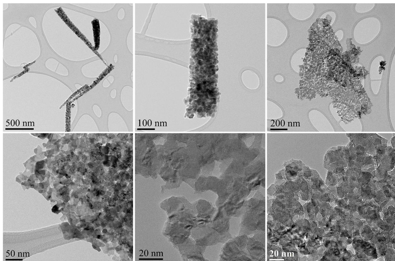
**Figure S6:** TEM images of NiCo<sub>2</sub>O<sub>4</sub>/PGR before OER experiments at different magnifications.
