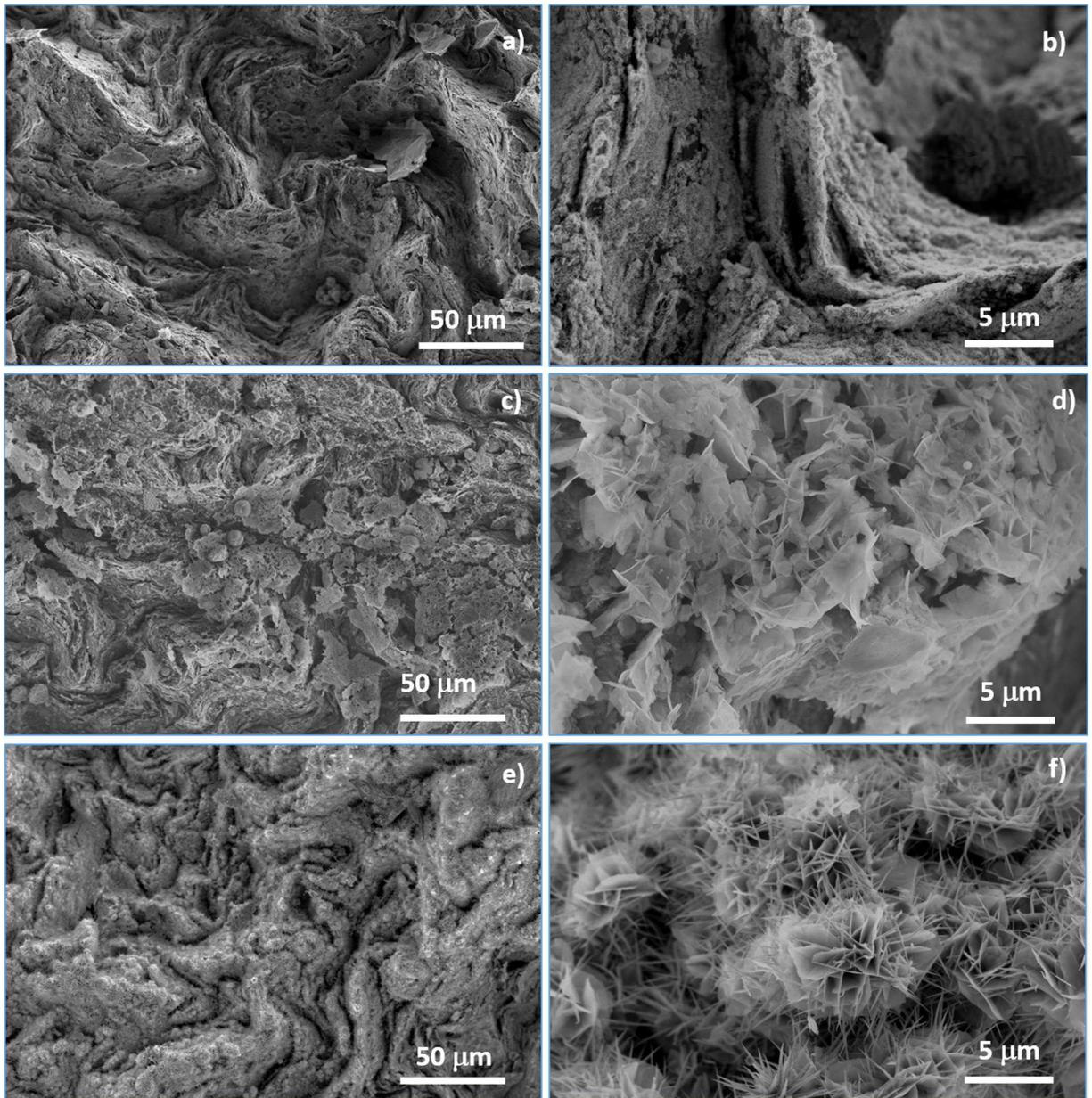
**Figure S2:** SEM images taken at different magnifications of the catalysts after their preparation: a) and b) NiO/PGR, c) and d)  $\text{Co}_3\text{O}_4$ /PGR and e) and f)  $\text{NiCo}_2\text{O}_4$ /PGR.
