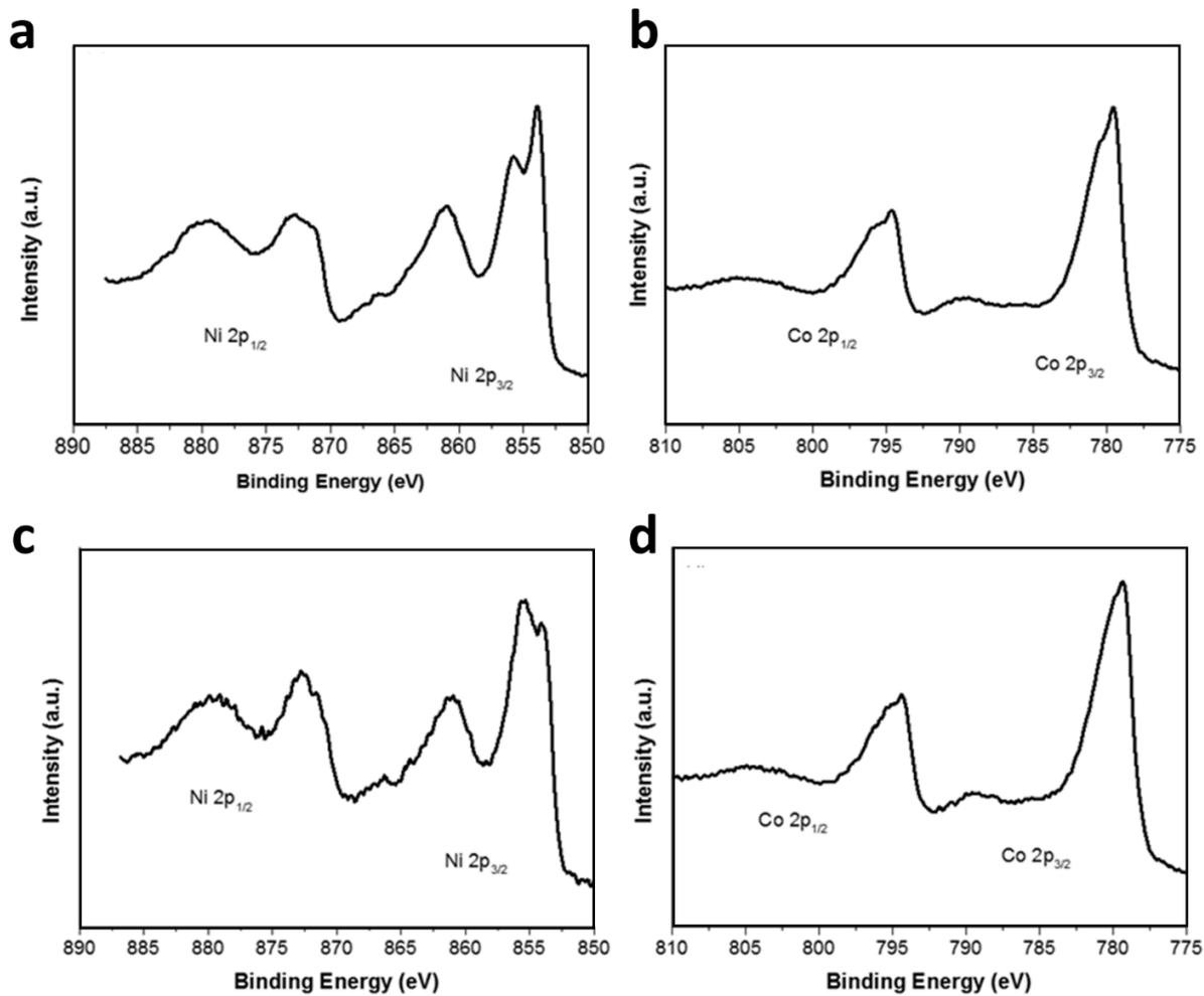
**Figure S5:** XPS spectra (a) Ni 2p of NiO/PGR; (b) Co 2p of Co<sub>3</sub>O<sub>4</sub>/PGR; (c) Ni 2p and (d) Co 2p of NiCo<sub>2</sub>O<sub>4</sub>/PGR.
