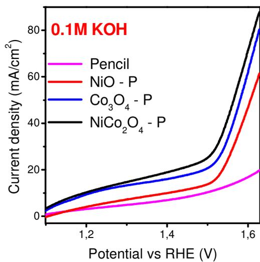
**Figure S9** . LSV curves of bare graphite pencil, NiO-P, Co<sub>3</sub>O<sub>4</sub>-P, NiCo<sub>2</sub>O<sub>4</sub>-P, at a scan rate of 5mVs<sup>-1</sup> in 0.1 M KOH
