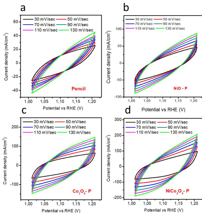
**Figure S8,** a. CV curves of bare graphite pencil at different scan rates in 1.0 M KOH, b. CV curves of NiO-P at different scan rate in 1.0 M KOH, c. CV curves of  $\text{Co}_3\text{O}_4\text{-P}$  at different scan rates in 1.0 M KOH, d. CV curves of  $\text{NiCo}_2\text{O}_4\text{-P}$  at different scan rates in 1.0 M KOH
