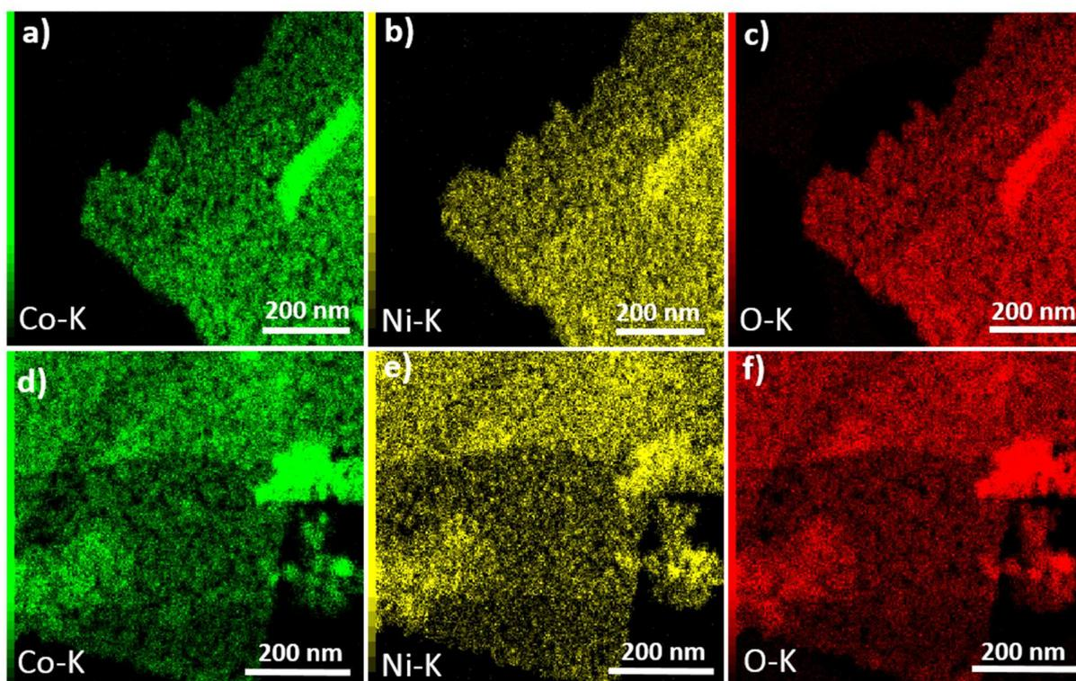
**Figure S7:** X-maps from EDS analyses of NiCo<sub>2</sub>O<sub>4</sub>/PGR before (a-c) and after (d-f) the OER reactions.
