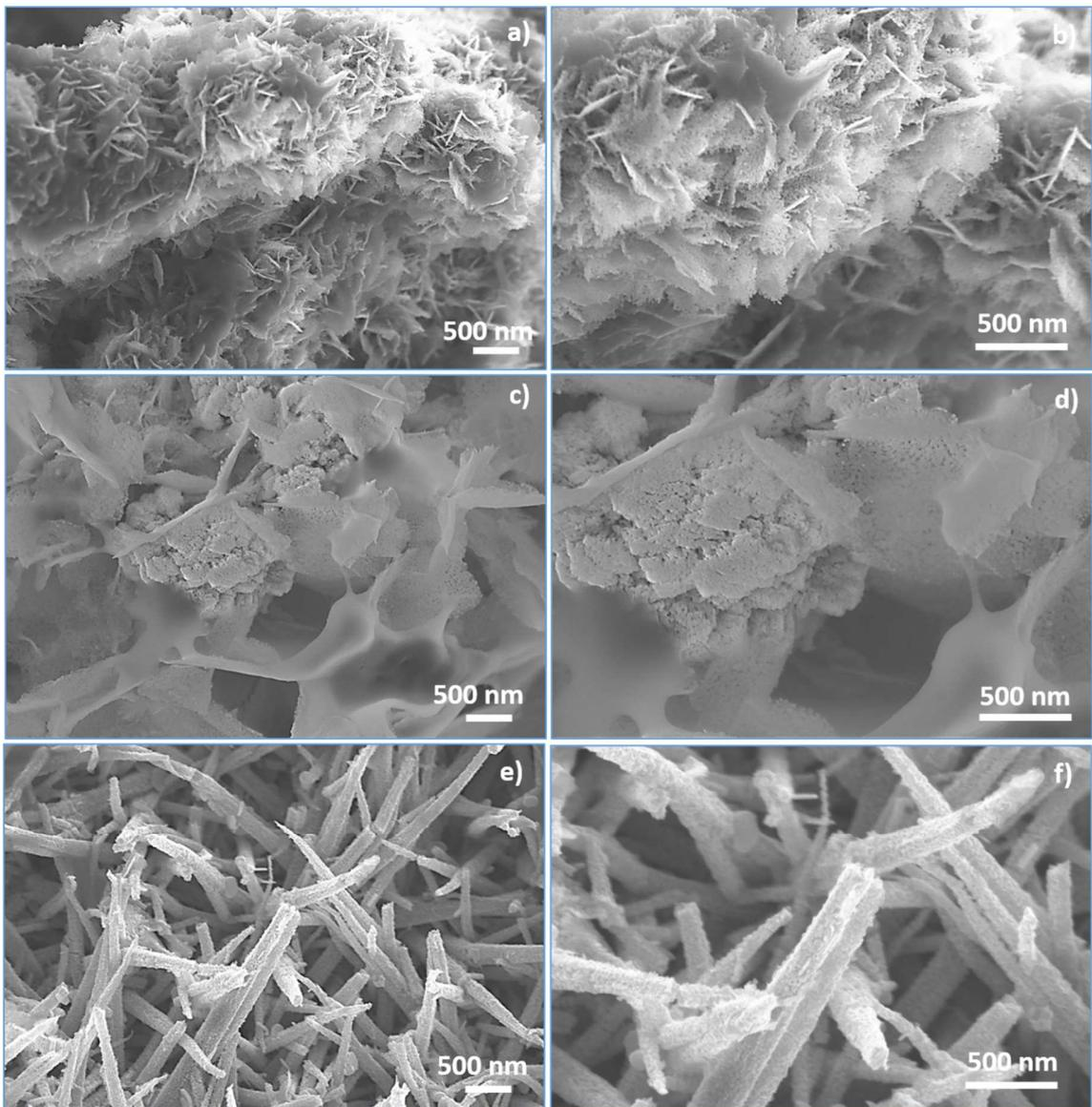
**Figure S3:** SEM images taken at different magnifications of the catalysts after OER experiments: a) and b) NiO/PGR, c) and d)  $\text{Co}_3\text{O}_4$ /PGR and e) and f)  $\text{NiCo}_2\text{O}_4$ /PGR.
