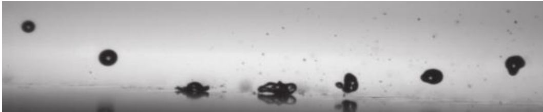
Fig. 3. Droplet-wall interaction in the bouncing regime (Weber < 40) [9]
