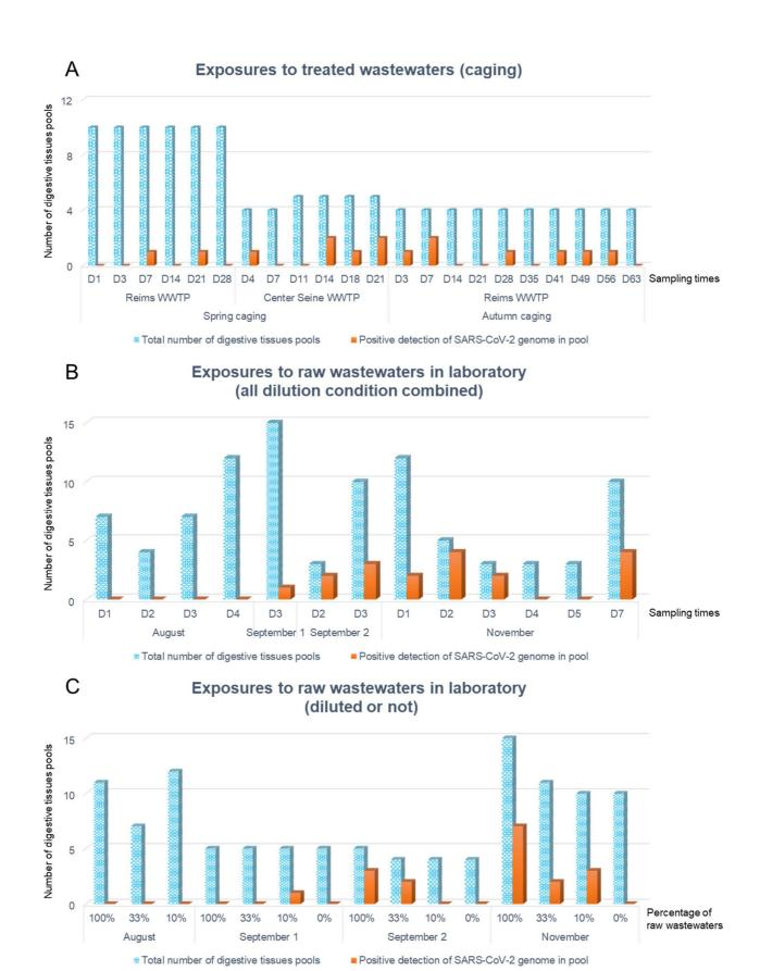
Figure 2: Total number of digestive tissues pool exposed (blue) and number of positive detections of SARS-CoV-2 genome in pools (orange) according to exposure, exposure condition and sampling times. A: Results obtained
