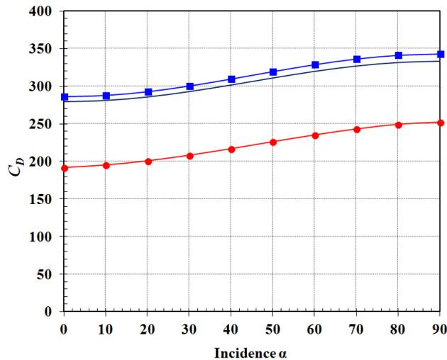
**Figure 2.** Drag coefficient obtained for the ellipsoid  $w=5/2$  at  $Re_p = 0.1$ . Present results: (—■—); theoretical results of Brenner [13]: (—); Results of Zastawny *et al.* [8] are also reported (—●—).
