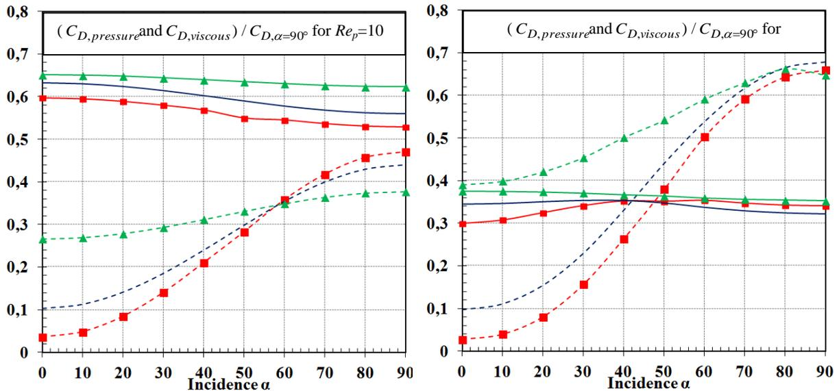
**Figure 5.** Pressure (dashed lines) and friction (continuous lines) drag coefficients versus  $C_{D,\alpha=90^\circ}$  as a function of the angle of incidence  $\alpha$  for different aspect ratios. (—■—):  $w=5/1$ ; (—●—):  $w=5/2$ ; (—▲—):  $w=5/4$ .
