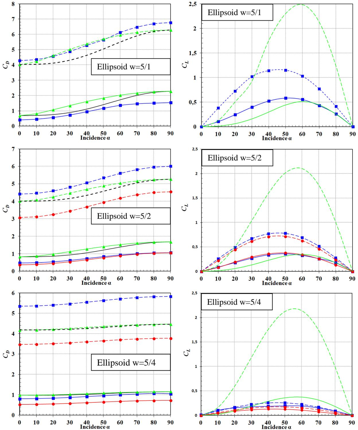
**Figure 3.** Comparison of the computed drag and lift coefficients with the existing correlations for different particles Reynolds numbers. On the left, drag coefficients and on the right lift coefficients as a function of the angle of incidence  $\alpha$ . (—): Rosendahl [7]; (—■): Ansys Fluent©; (—●): Zastawny *et al.* [8]; (—▲): Hölzer & Sommerfeld. [5]; (—): Hoener. [10]. The dashed lines are referred to  $Re_p = 10$  and the continuous lines are referred to  $Re_p = 300$ .
