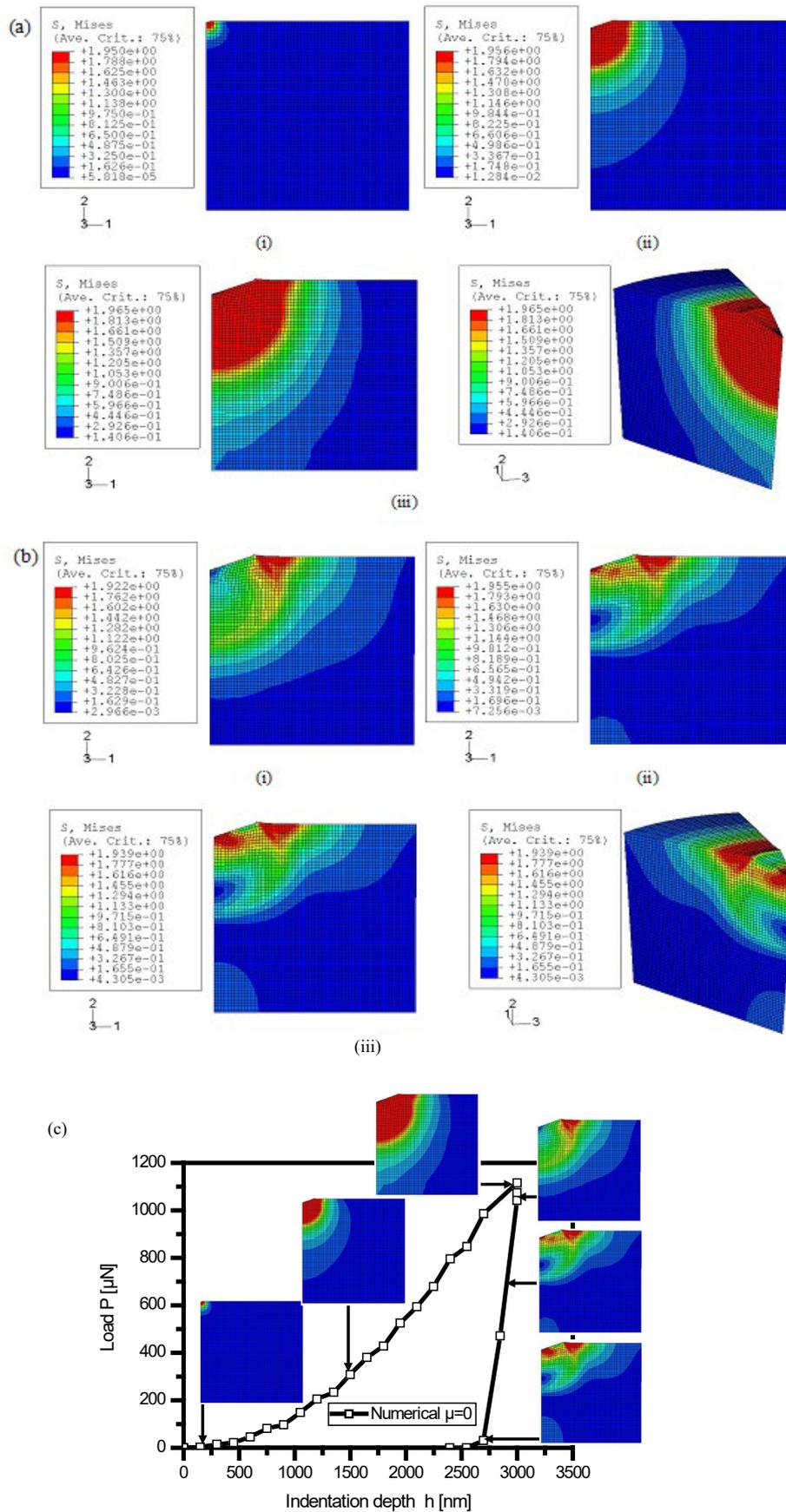
**Figure 8.** Contour of the Von Mises stress at different indentation depths: (a) loading part only, with (i)  $h = 50$  nm; (ii)  $h = 1500$  nm; (iii)  $h = 3000$  nm; (b) unloading part only, with (i)  $h = -50$  nm; (ii)  $h = -1500$  nm; (iii)  $h = -3000$  nm; (c) Numerical load–displacement curves and corresponding, predicted, specimen shapes
