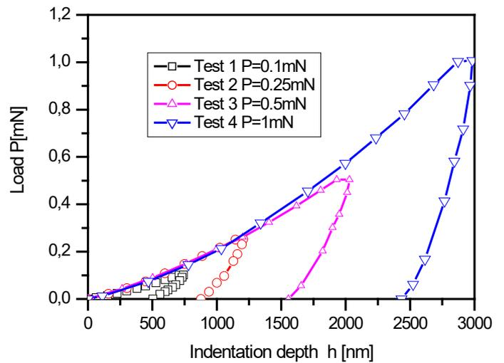
Figure 3. Experimental load-displacement curves at different loads indicated in the inset, leading to four different indentation depths
